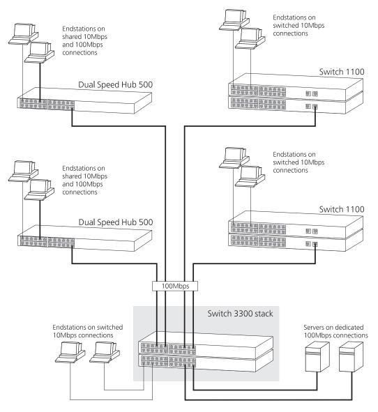
..... ..... Switch 3300 as a Desktop Switch The example in Figure 5 shows how a Switch 3300 can be used for a group of users that require dedicated 10Mbps or 100Mbps connections to the desktop. The Switch 3300 stack has a SuperStack II Switch 1000BASE-SX Module that allows it to provide a Gigabit Ethernet link to a SuperStack II Switch 9000 SX in the basement.
