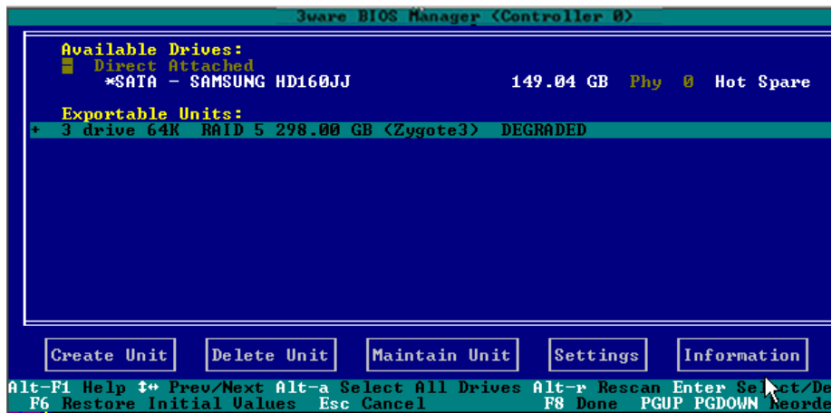
Figure 65. Degraded RAID 5 Array to be Rebuilt
