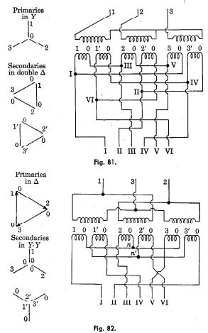
employed when synchronous converters are used to supply power for electrical railways. The double-Y connection is always used when a neutral is desired for grounding or for the neutral wire of a three-wire d-c system which receives power from a six-phase synchronous converter. The primaries should be connected in  $\Delta$  when the diametrical connection is used for the secondaries because of the suppression of the third-harmonic components in the exciting currents by Y-connected primaries.
