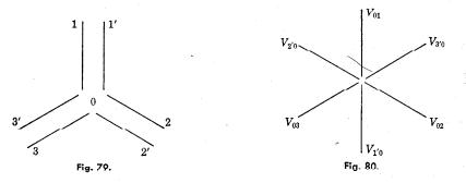
secondaries are connected in  $\Delta$  to give a closed path for the third harmonic of the exciting current which is suppressed in the primaries by Y, connection. The two sets of secondaries are connected to form two independent three-phase systems with the connections of one set of secondaries reversed with respect to the connections of the other set.
