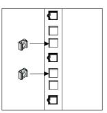
4. Align the mounting holes on the top bracket with the caged nuts you installed in Step 3, and insert two mounting screws (provided with the enclosure) to secure the top bracket.
