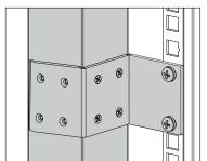
5. Repeat Step 4 for the bottom bracket to secure the strip to the enclosure.
