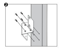
2. Choose a suitable location for the strip. The figure at right shows the strip mounted in four different locations in the enclosure. To avoid interfering with shelves or equipment, install the strip so that it hangs on the outside edge of the vertical rail.
