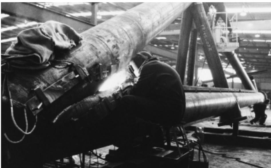
Figure 2. Shop fabrication of some of the large tubular trusses used in the Colonial Stadium.
