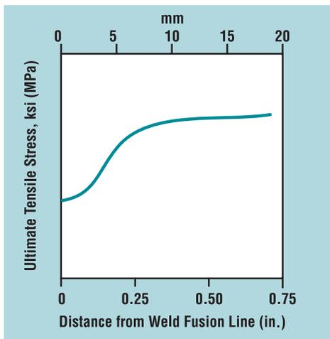
Figure 4. Tensile stress vs. distance from weld fusion line.
