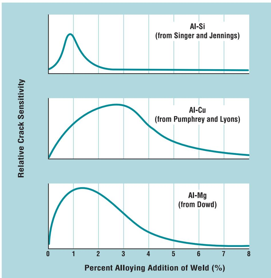
Figure 1. Relative crack sensitivity versus weld composition for various binary aluminum systems.
