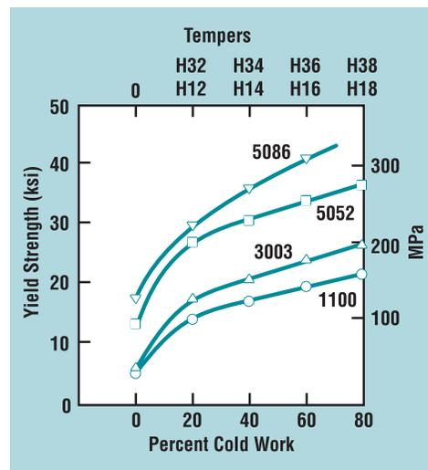
Figure 3. Effect of cold work on yield strength of several work-hardening alloys.
