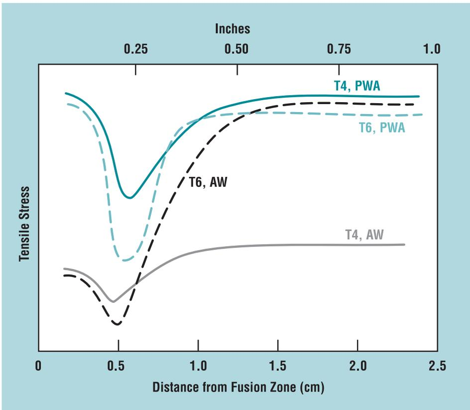
Figure 5. Tensile stress profiles of the heat affected zone for 6061-T4 and T6 starting material in the As-Welded (AW) and Post-Weld Aged (PWA) conditions.
