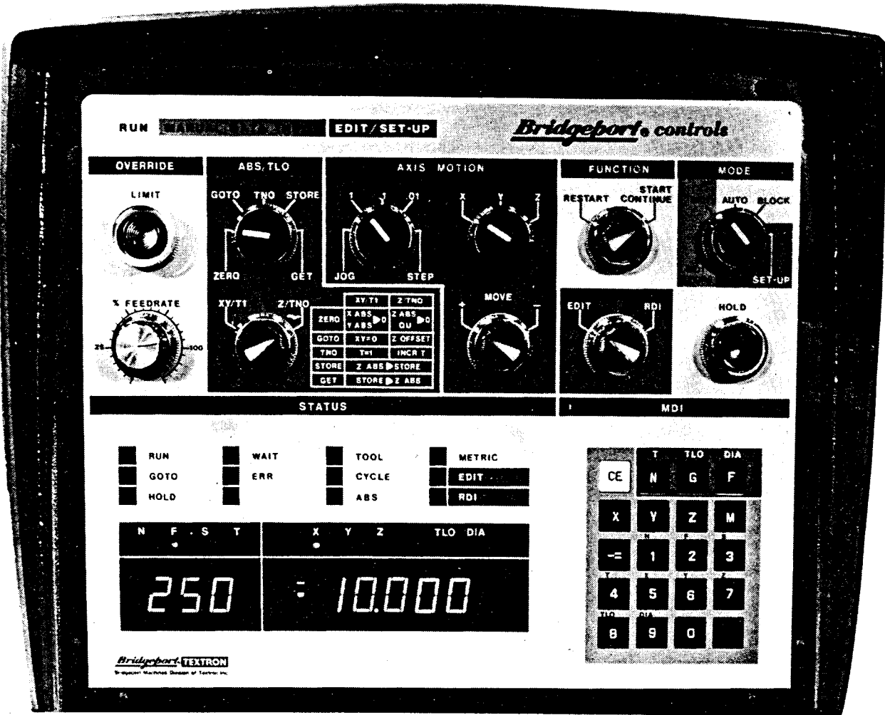
OPERATOR'S MAIN CONTROL PANEL
