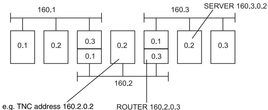
The boxes represent for example TNCs or personal computers. Please observe that a TNC can never be a ROUTER, since it does not feature the second connector for feeding signals through.
