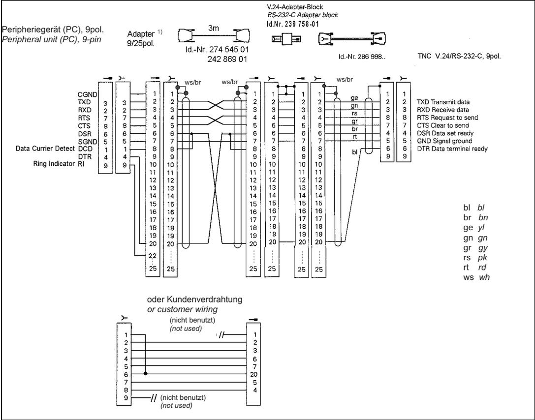
1) Customer wiring or prefabricated part
