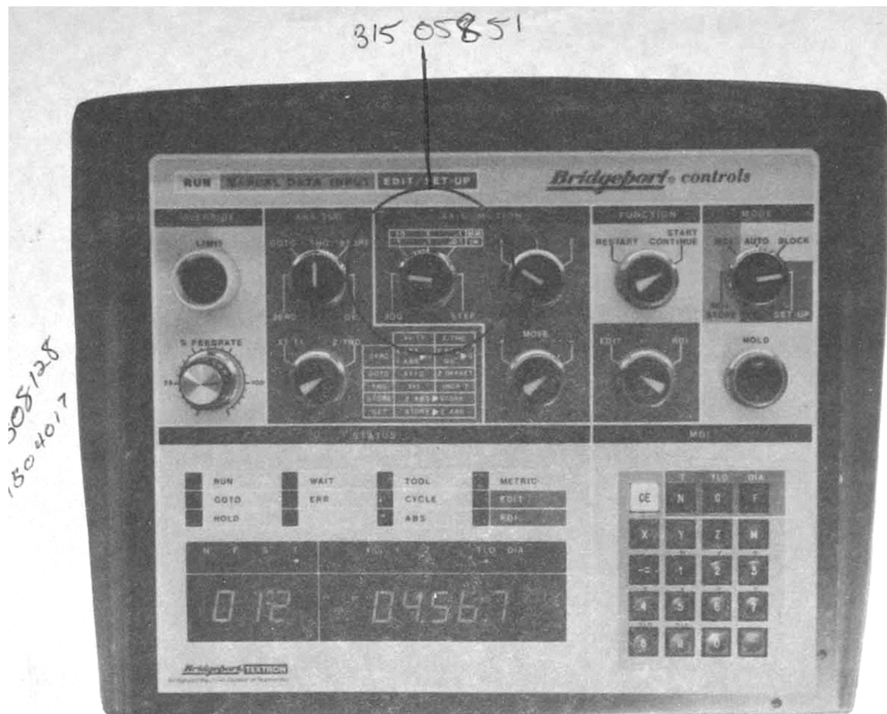
Figure 4-2 Operator's Main Control Panel S/N 7410 and After
