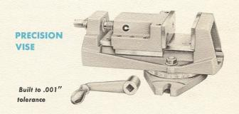
Surfaces of hardened jaw and slide plates are ground flat and parallel to within .001" — top and bottom of bed and swivel base are ground flat and parallel to within .001". Jaw plates are 4" wide, 13/4" high, open 3". Swivel base graduated 0° to 90° both directions. Crank is forged steel.
