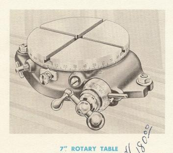
Precision built for accurate, angular indexing and spacing operations. Ground table is graduated 0° to 90° in each quadrant, has T-slots for 5/16" bolts, positive lock, crank with graduated friction-clutch dial and throw-out for free table movement. Table and dial graduations easily synchronized. Provision for take-up provided.
