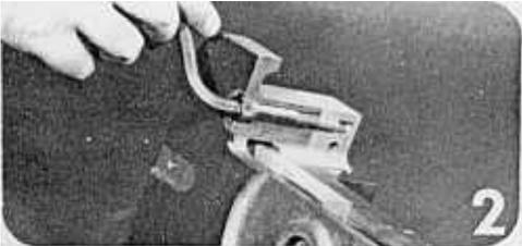
Remove the two socket head cap screws holding the stationary jaw to the bed.
