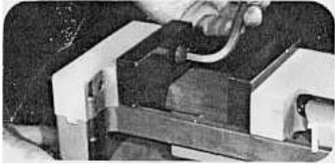
If your vise should become worn or abused where repairs are required, note the simplicity required to restore the vise to new condition even in your own shop. First, note that the jaw plate can easily be removed.
