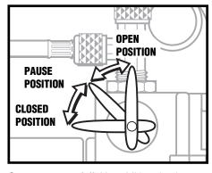
Quarter-turn on/off. No additional valve needed to isolate system.
