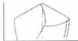
Plus (+) setting (more relief, turn counter-clockwise)
