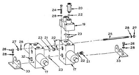
Figure 12 - Exploded View Of Valve Bank
