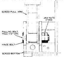
Detailed Of Screed Hinge Bolt In-place Figure 35).
