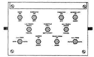
Figure 7 - Paver Control Console
