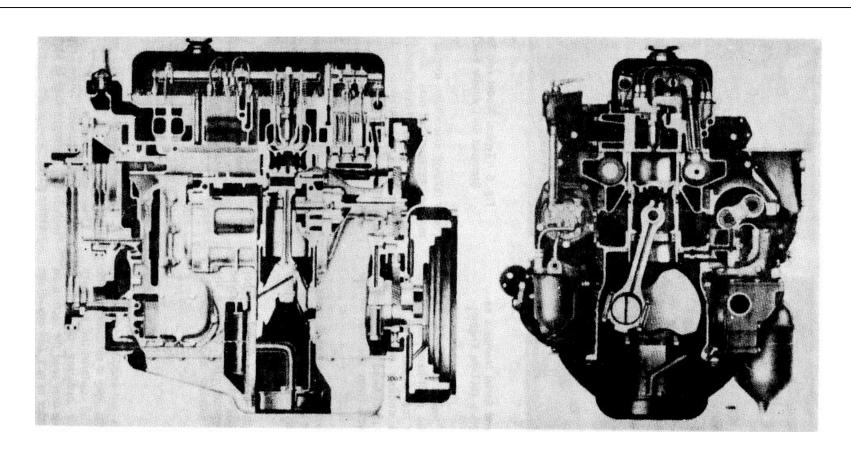
Cross Section Views of a Typical In-Line Engine
