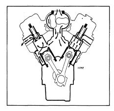
Fig. 7 - Air Intake System Through Blower and Engine (6V-53 Engine)
