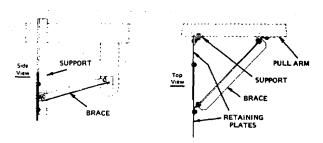
Typical 36" Retaining Plate Arrangement Figure 16
