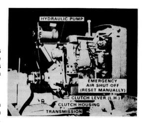
Figure 9. Detroit Diesel Engine (Cover Removed)
