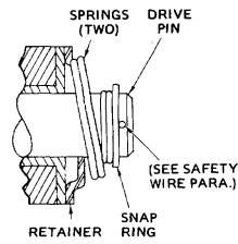
Detail Of Brake Auto-gap Drive Pin Figure 42
