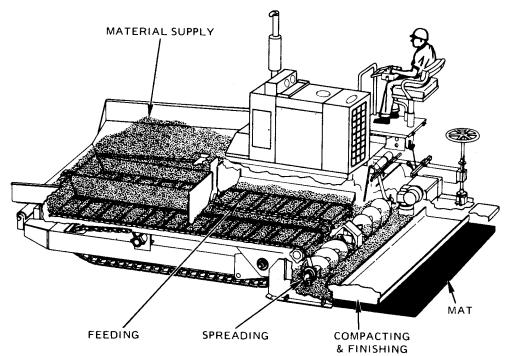
Figure 9. Material Flow Diagram
