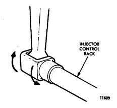
Fig. 4 · Checking Rotating Movement of Injector Control Rack
