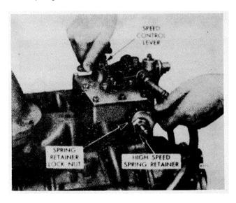
Fig. 6 - Adjusting Maximum No-Load Engine Speed
