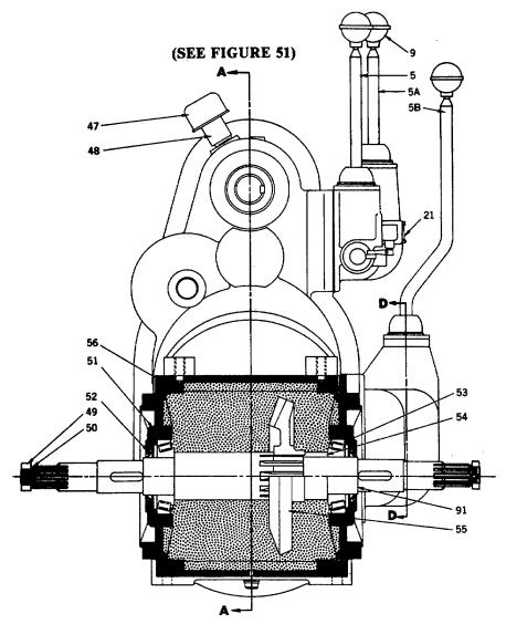
End View Cut-away of 24 Speed Manual Shift Transmission (View B-B, Figure 51) Figure 52
