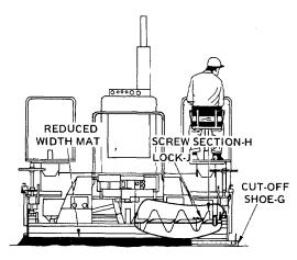
Laying Reduced Width Mat Using
