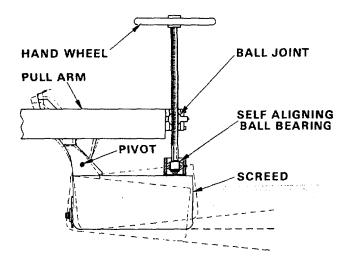
Effect of Handwheel Adjustment on Screed Figure 5
