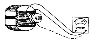
Resistance of Field Circuits at 25°C -(77°F)
