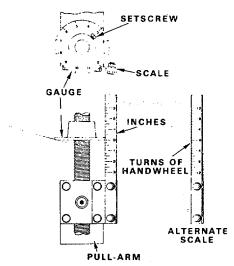
Handwheels Set to Level Inclined Roadway Figure 6
