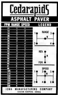
Figure 8. 24-Speed Transmission
