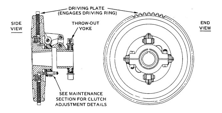
Figure 5. Friction Clutch- Main Drive
