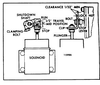
Fig. 6 - Typical Speed Governor Lever Position
