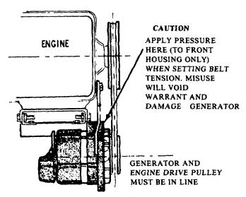
Correct Alignment of Generator Pulley Figure 60
