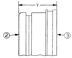
Side View Brake Showing Wear-check Dimension Figure 45
