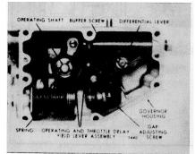
Fig. 4 - Throttle Delay Yield Lever (6V Engine)
