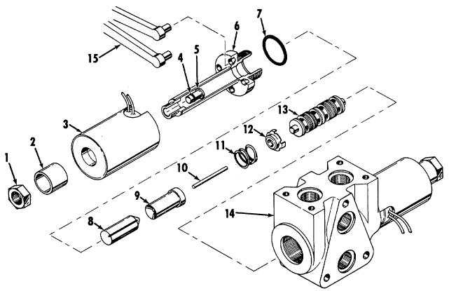
Figure 10 - 4 Way Solenoid Operated Hydraulic Valve - Exploded View
