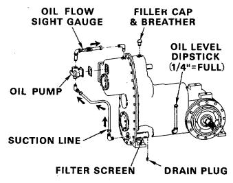
Transmission Oiling System - Exploded View
