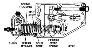
Fig. 6 - Location of Shims and Stops
