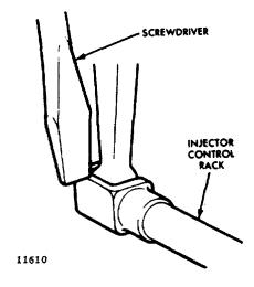
Fig. 4 - Checking Injector Control Rack "Spring"
