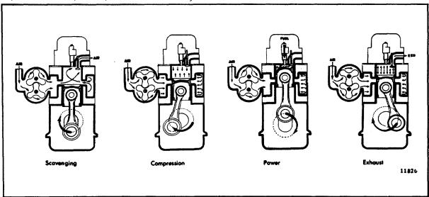
Fig. 1 - The Two-Stroke Cycle
