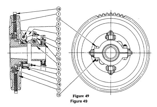
**COMPOPNENT PARTS IDENTIFICATION - TWIN DISC C-110 CLUTCH**
