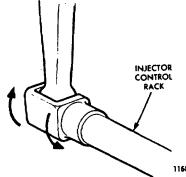
Fig. 3 - Checking Rotating Movement of Injector Control Ra
