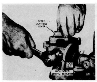
Fig. 5 - Adjusting Maximum No-Load Engine Speed (Type A)
