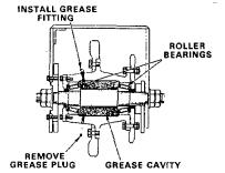
Cross-section thru Track Sprocket Figure 7
