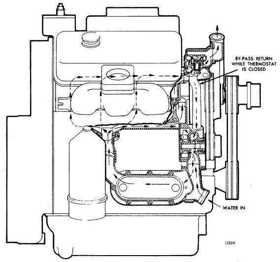
Fig. 19 - Typical Cooling System for V-Type Engine
