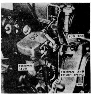
Fig. 1-Hydraulic Governor mounted on Engine
