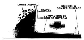
Cross-section thru Screed and Material Figure 2
