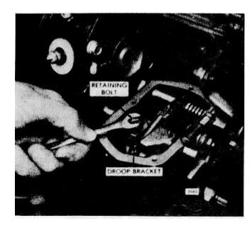
Fig. 3 - Adjusting Length of Fuel Rod
