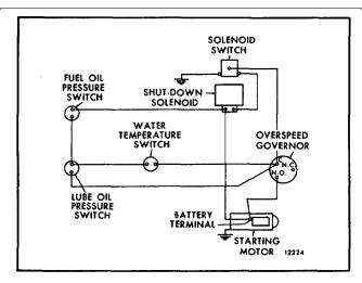
Fig. 3. - Automatic Electrical Shut-Down System Diagram.
