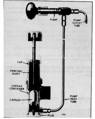
Fig. 8 - Typical Fluid Starting Aid
