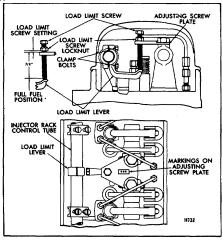
Fig. 1 - Engine Load Limit Device
