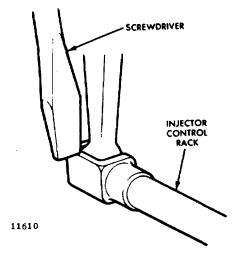
Fig. 5 - Checking Injector Control Rack Spring
