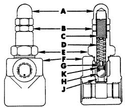
Figure 15 - Pressure Relief Valve - Cross Section
