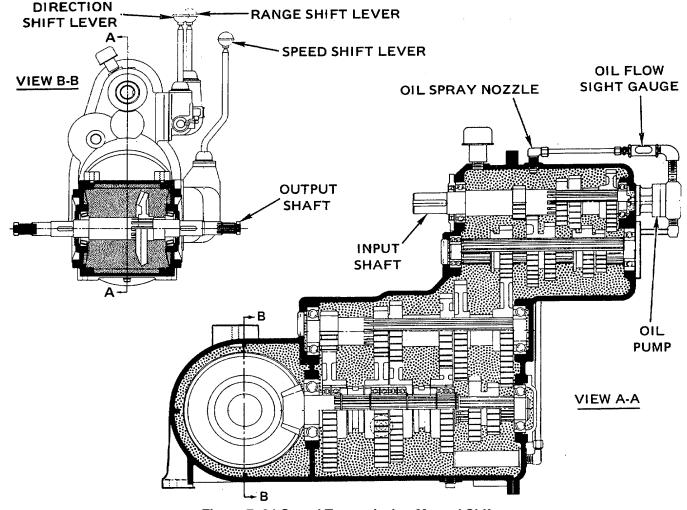
Figure 7. 24 Speed Transmission-Manual Shifts
