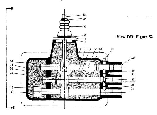
Side & End View Cross-sections Of 6 Speed Shift Lever Module Figure 54
