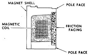
Cross-section Thru Electric Brake Magnet Assembly Figure 46
