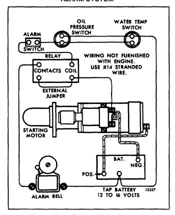
Fig. 5 - Alarm System Wiring Diagram.
