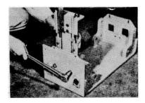
**9.** Install the capscrews which attach the Strike\* off Plate to the Adjusting Bolts. Tighten the screws.
