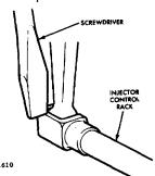
Fig. 5 - Checking Injector Control Rack "Spring"
