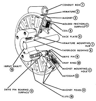
Cut-away Showing Electric Brake Components Figure 41
