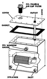
Figure 6 - Reservoir - Exploded View
