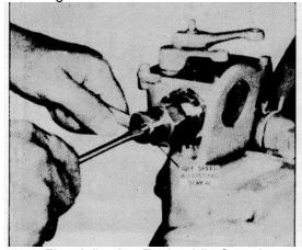
Fig. Adjusting Engine Idle Speed
