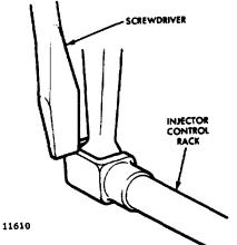
Fig. 4 - Checking Injector Rack "Spring"
