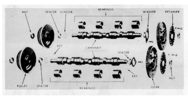
**CAMSHAFT AND GEAR (V-ENGINE)**
