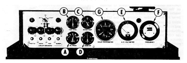
Figure 1. Instrument Panel - (Protective Cover In Unlocked Position)
