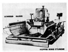
Figure 19 - Tilting Hopper Wings
