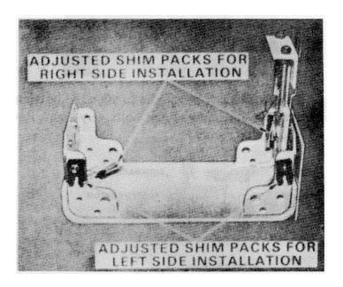
Extension With Adjusted Shim Packs Attached Figure 30
