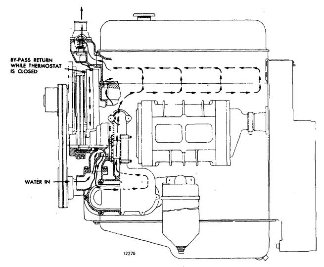
Fig. 18 • Typical Cooling System for In-Line Engines
