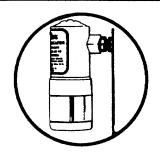
1 Measure the restriction of the air cleaner with a Donaldson restriction indicator, service gauge, or a water manometer at the restriction tap provided in the air cleaner, the transfer pipe, or the blower intake. Replace or clean the element only when the restriction has reached the maximum allowed by the engine or equipment manufacturer.
