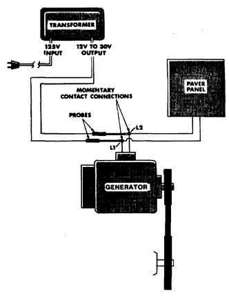
Method Of Flashing 125 V AC Generator Figure 56
