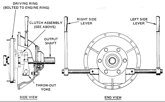
Figure 6. Dual Throw-Out Control For Main Drive Clutch
