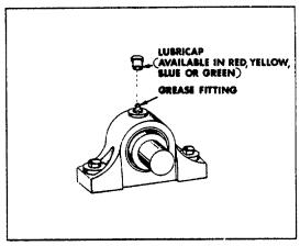
Plastic Lubricap for Bearing Grease Fittings Figure 2
