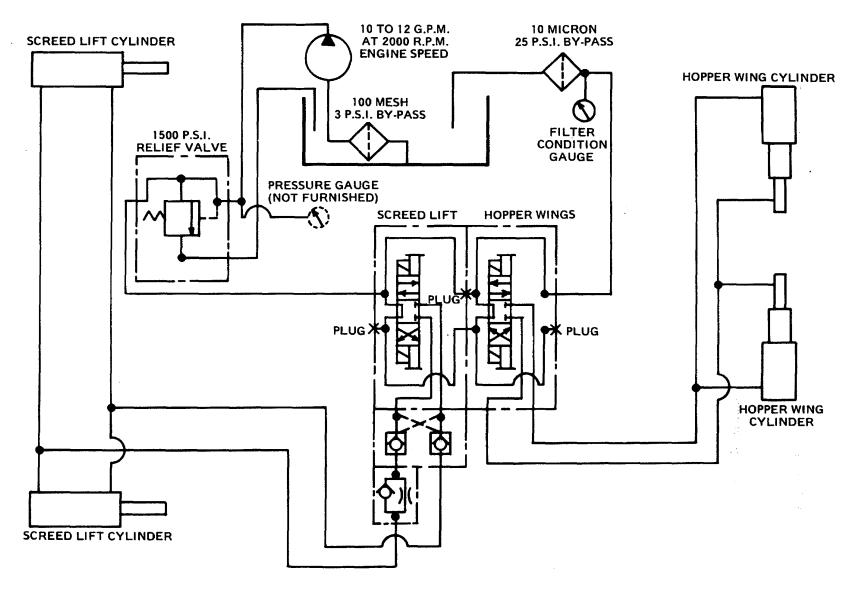
Schematic Diagram-BSF-400 Paver Hydraulic System Figure 23
