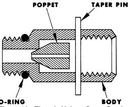
Figure 16 - Throttle Valve - Cross Section
