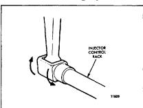
Fig. 4 - Checking Rotating Movement of Injector Control Rack
