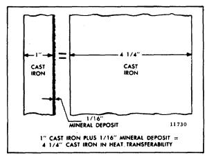
Fig. 2 - Heat Transfer Capacity
