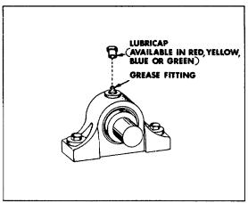
Plastic Lubricap for Bearing Grease Fittings
