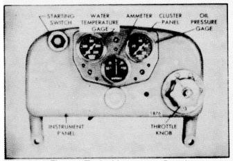
Fig. 1 - Typical Instrument Panel
