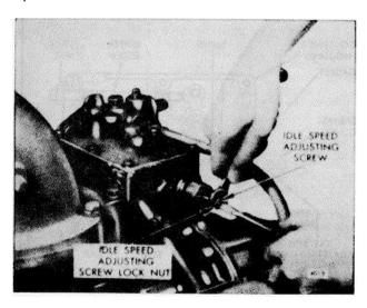
Fig. 8 - Adjusting Engine Idle Speed
