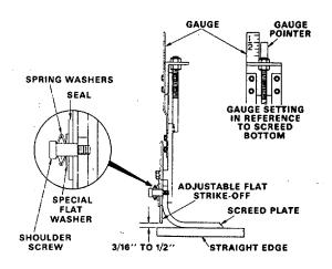
Cross-section - Flat Strike-off Assembly Figure 25
