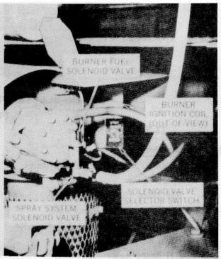
Screed Burner Solenoid Valves & Switch Figure 9
