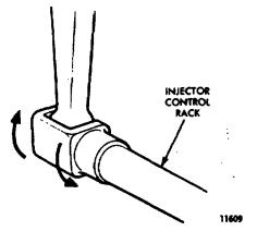
Fig. 3 - Checking Rotating Movement of Injector Control Rack
