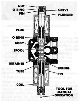
Figure 9 - Solenoid Valve - Cross Section
