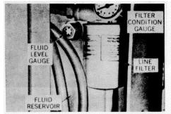
Figure 5 - Line Filter & Filter Condition Gauge
