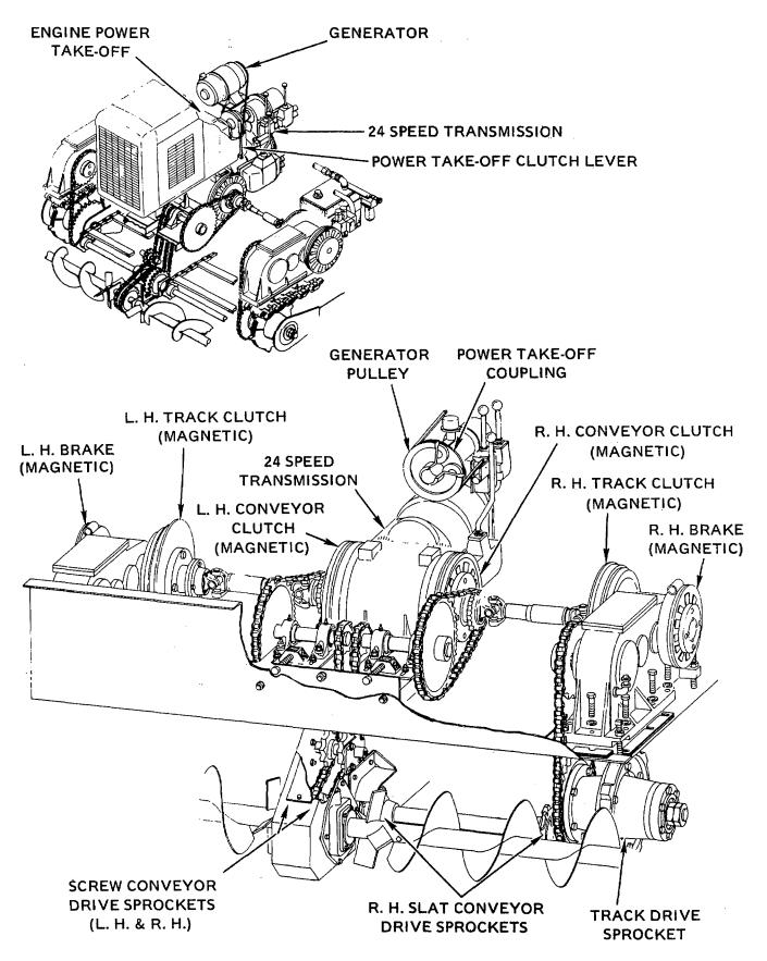
Figure 4. Travel & Conveyor Drive Arrangements
