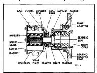
Fig. 20. - Raw Water Pump Used on In-Line Engine.
