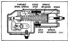
Fig. 5 - Locating of Shims and Stops
