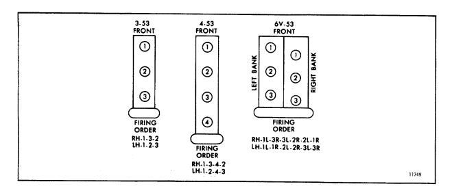
Fig. 4. Series 53 Cylinder Arrangement
