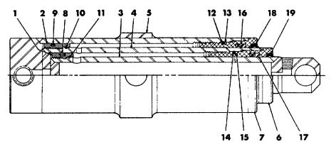
Typical Hopper Wing Cylinder — Double Acting, Double Stage Type
