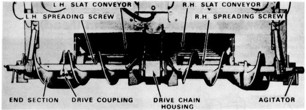
Slat Conveyors and Spreading Screws (Screed Removed)
