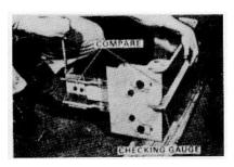
**11.** Use gauge tool to check accuracy of Gauge and Pointer read-out when strike-off plate is raised.
