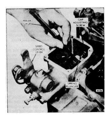
Fig. 1 - Checking Governor Gap
