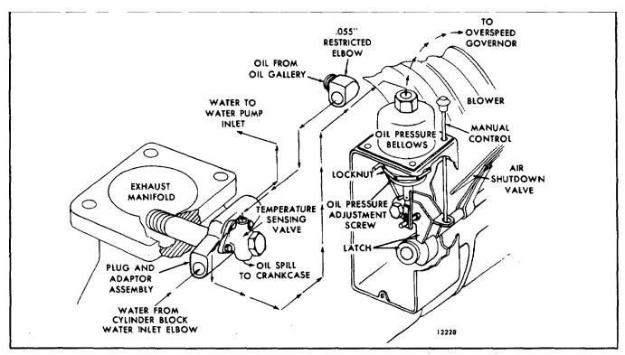
Fig. 2 - Mechanical Shutdown System Schematically Illustrated.
