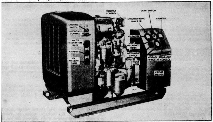
Fig. 1 - Location of Controls on Power Generator Set
