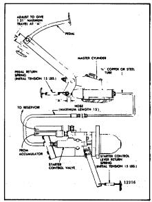
Fig. 7 - Hydrostarter Remote Control System
