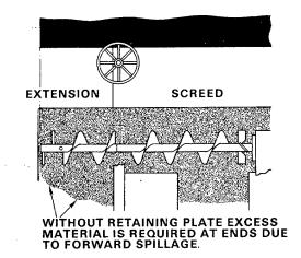
Paving with Extensions - No Retaining Plate Figure 10
