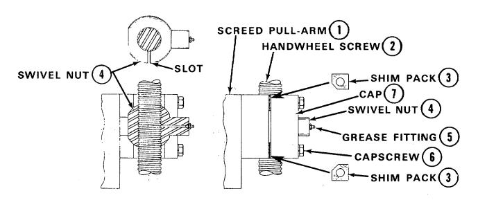
Detail Of Screed Handwheel Screw And Pull-arm Swivel Nut Coupling Figure 36
