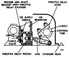
Fig. 2 - Throttle Delay Cylinder
