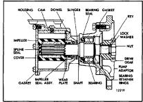
Fig. 21. - Raw Water Pump Used on V-Type Engine.
