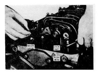
Fig. 2 - Adjusting Valve Clearance (Four-Valve Cylinder Head)
