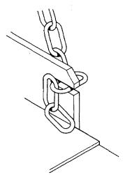
Method of Attaching Chain for Bleeding
