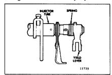
Fig. 3 - Throttle Delay Yield Lever (In-Line Engine)
