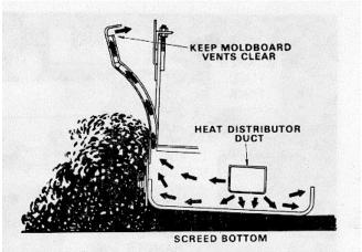
Cross-section Showing Heat Flow Thru Screed Figure 32
