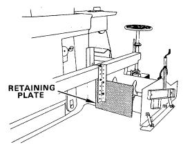
Retaining Plate used with Screed Extension Figure 9
