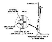
**8.** Arrange the Seal and the three Washers on each Shoulder Screw as shown above
