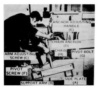
Adjusting Side Plate Chain Anchor Figure 13
