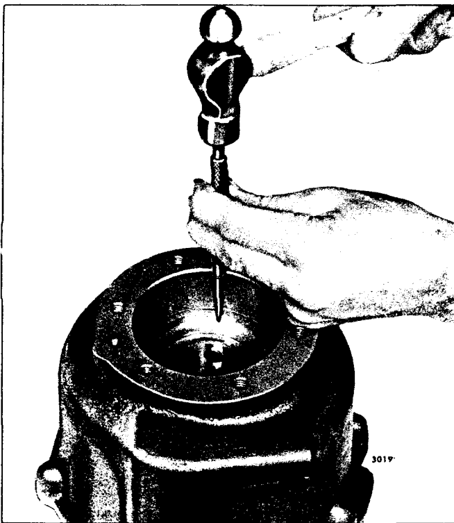
Fig. 38 - Removing Roll Pin from Sun Gear Dowel Pin (1.5:1 Ratio)
