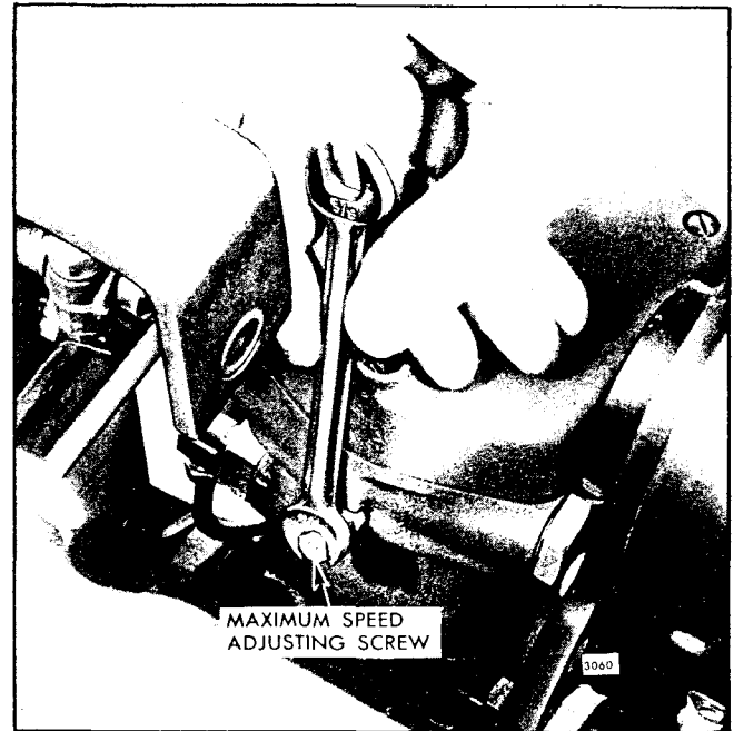
Fig. 5 - Adjusting Maximum Engine Speed
