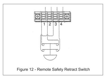
For added protection of the user, a terminal strip is located on the electric panel allowing easy installation of a remote safety retract switch.
