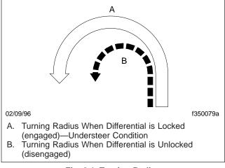
Fig. 9.1, Turning Radius
