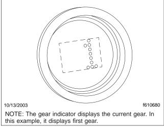
Fig. 8.26, Current Gear Display
