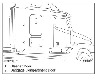
Fig. 3.5, Passenger-Side Sleeper and Baggage Compartment Doors
