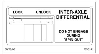
Fig. 2.35, Interaxle Differential Lockout Switch
