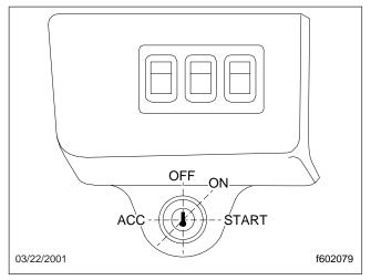
Fig. 7.6, Ignition Switch Positions
