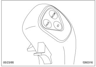
Fig. 2.20, Cruise Control, Transmission Shift Knob Buttons
