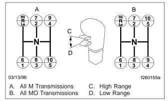
Fig. 8.16, Meritor 10-Speed Transmission Shift Patterns
