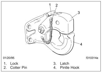
Fig. 10.22, Holland PH-T-60-AL Trailer Coupling
