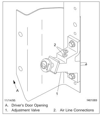
Fig. 2.26, Tilt Steering Wheel Control Pedal
