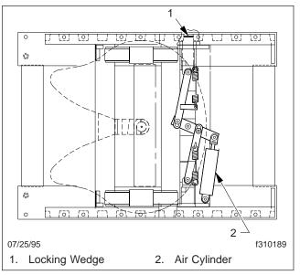
Fig. 10.14, Air-Operated Sliding Fifth Wheel Mount, AWB Model
