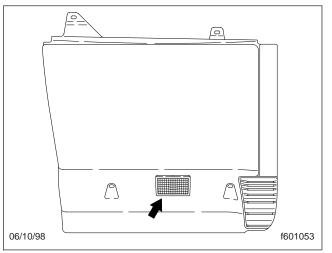
Fig. 2.41, Passenger's Footwell Courtesy Light
