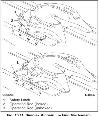
Fig. 10.11, Simplex Kingpin Locking Mechanism, Locking and Unlocking
