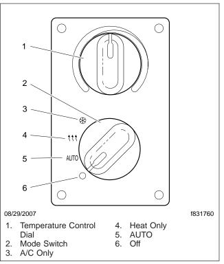
Fig. 4.6, Parked A/C and Heater Control Panel
