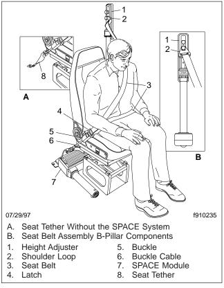
Fig. 5.13, SPACE System Seat Belt Assembly
