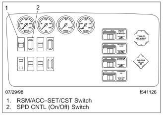
Fig. 2.19, Cruise Control Switches, Dash-Mounted
