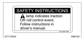
Fig. 2.48, Roll Stability Control Dash Decal
