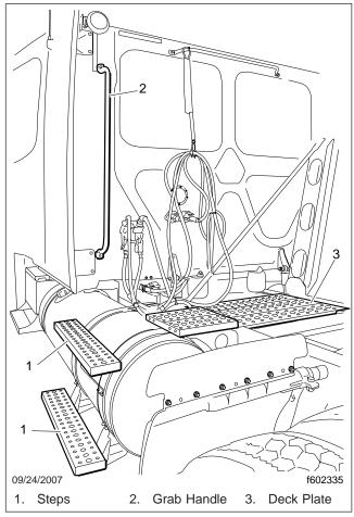
Fig. 3.6, Back-of-Cab Access
