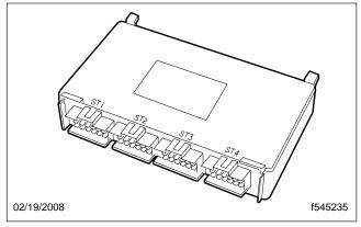
Fig. 2.25, Common Powertrain Controller (CPC)
