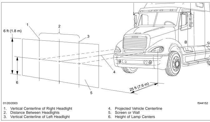
Fig. 14.1, Headlight Aiming Screen or Wall
