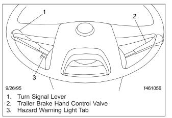
Fig. 6.2, Steering Column-Mounted Controls (left-hand drive shown)
