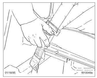
Fig. 5.9, Releasing the Three-Point Seat Belt
