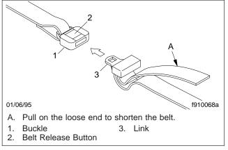
Fig. 5.10, Bunk Restraint Adjustment
