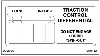
Fig. 2.34, Controlled Traction Differential Switch
