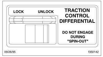
Fig. 9.3, Traction Control Differential Control
