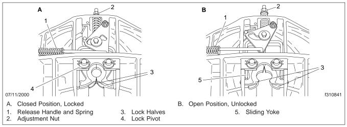
Fig. 10.4, Type "B" Kingpin Lock Mechanism (bottom view)
