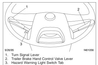
Fig. 2.29, Steering Column-Mounted Controls
