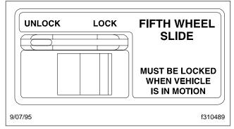
Fig. 2.36, Fifth Wheel Air Slide Switch
