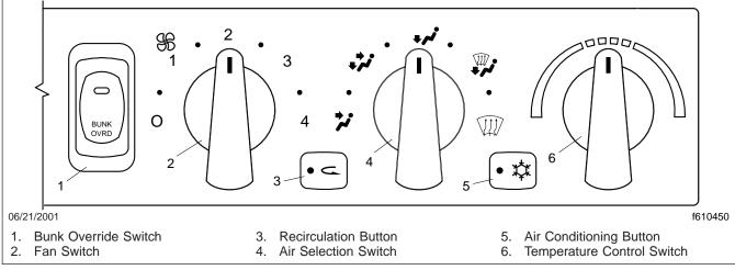
Fig. 4.1, Cab Climate Control Panel
