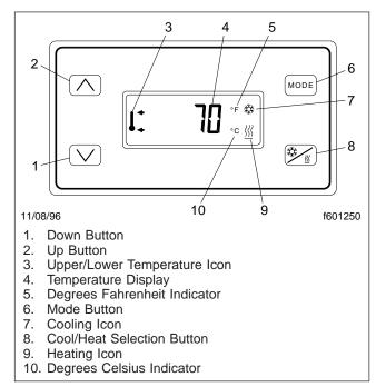
Fig. 2.23, Optimized Idle Thermostat
