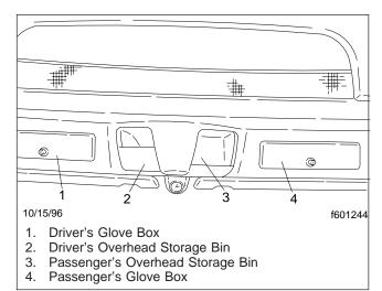
Fig. 3.8, Glove Boxes and Overhead Storage
