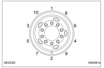
Fig. 11.7, Tightening Pattern, 10-Hole Wheels
