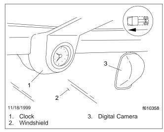
Fig. 2.47, Lane Departure Warning System Camera
