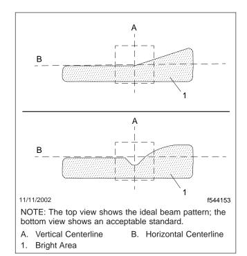
Fig. 14.3, Headlight Beam Patterns
