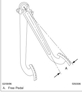
Fig. 7.8, Clutch Free Pedal Travel
