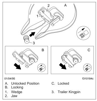
Fig. 10.16, Fontaine Kingpin Lock Mechanism
