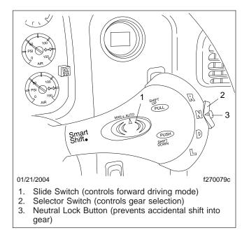
Fig. 8.25, Switches, UltraShift Transmissions
