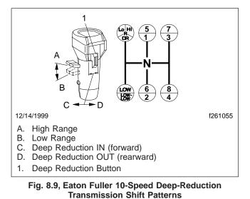
NOTE: The 3rd/7th and 4th/8th shift positions in the RT and RTX-LL transmissions are opposite of the RTO-LL transmissions.
