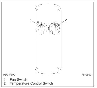
Fig. 4.5, Sleeper Climate Control Panel
