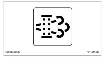
Fig. 7.2, Diesel Particulate Filter (DPF) Status Lamp
