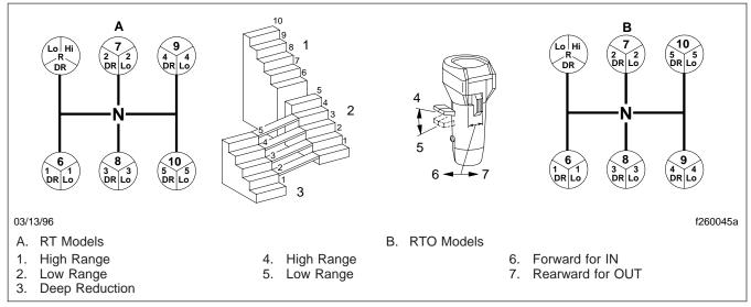
Fig. 8.10, Eaton Fuller 15-Speed Deep-Reduction Transmission Shift Patterns
