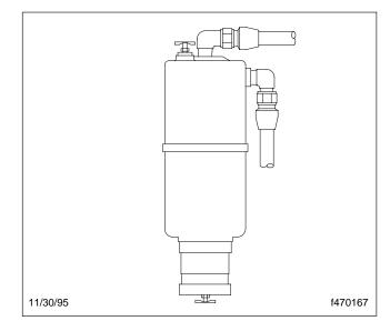
Fig. 11.3, ConMet Fuel/Water Separator
