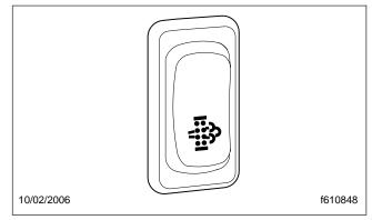
Fig. 2.33, Request/Inhibit Regen Switch
