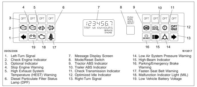
Fig. 2.4, ICU4-2 Dash Message Center (typical), EPA07 Compliant
