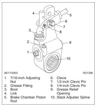
Fig. 11.10, Gunite Automatic Slack Adjuster
