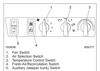
Fig. 2.28, Heater/Air Conditioner Controls
