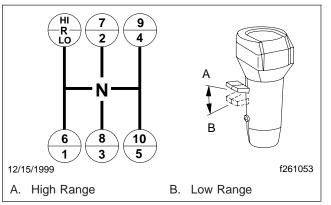
Fig. 8.6, Eaton Fuller 10-Speed Transmission Shift Patterns
