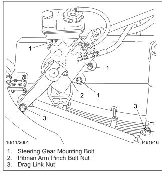
Fig. 11.12, Steering Gear Fasteners
