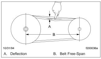
Fig. 11.13, Checking Belt Tension
