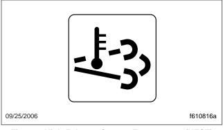
Fig. 7.1, High Exhaust System Temperature (HEST) Lamp
