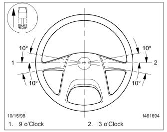
Fig. 6.1, Proper Steering Wheel Position (with tires pointed straight ahead)
