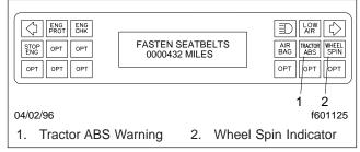
Fig. 2.44, ABS Warning and Indicator Lights (standard)
