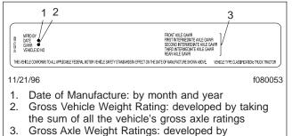
considering each component in an axle system including suspension, axle, wheels, and tires - and using the lowest component capacity as the value for the system
