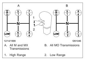
Fig. 8.15, Meritor 9-Speed Transmission Shift Patterns
