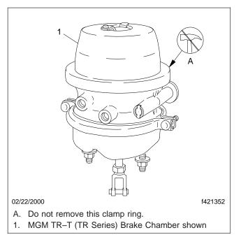
Fig. 11.9, Parking Brake Chamber Clamp
