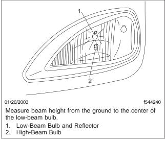
Fig. 14.2, Headlight Beam Height
