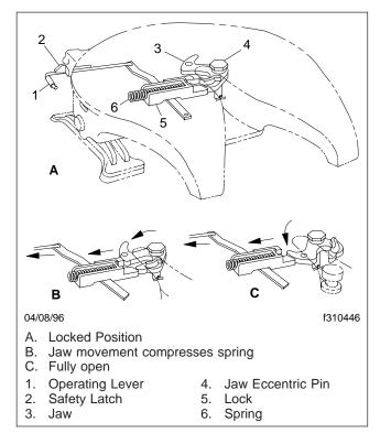
Fig. 10.10, ASF Simplex Series Kingpin Locking Mechanism Operation
