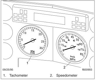
Fig. 2.15, Instrument Panel, Level II (center)
