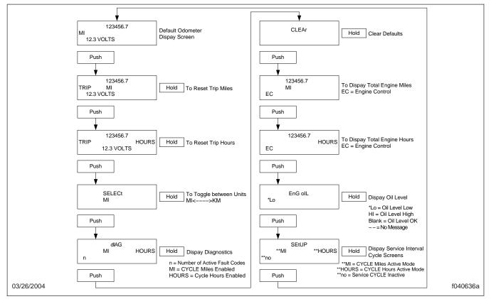
Fig. 2.12, ICU3/ICU3 '07 Mode Reset LCD Display Cycle
