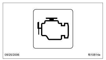
Fig. 7.4, Malfunction Indicator Lamp (MIL)
