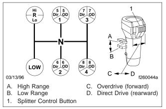
Fig. 8.7, Eaton Fuller 13-Speed Transmission Shift Pattern
