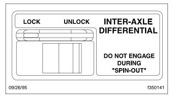
Fig. 9.4, Interaxle Differential Control
