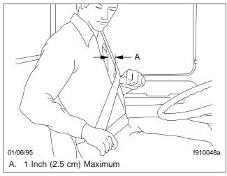
Fig. 5.7, Adjusting Shoulder Harness Clearance
