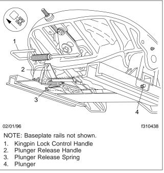
Fig. 10.3, Manual Release Slide
