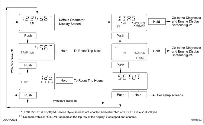
Fig. 2.5, ICU4/ICU4-2 Mode/Reset Switch Basic Functions
