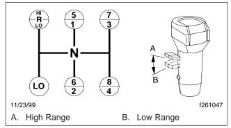
Fig. 8.5, Eaton Fuller 9-Speed Transmission Shift Patterns
