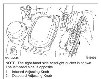
Fig. 14.4, Headlight Adjusting Knobs
