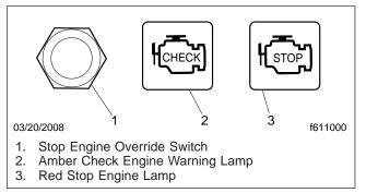
Fig. 2.1, Engine Lamps
