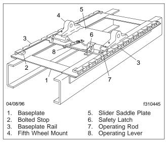
Fig. 10.9, Taperloc Slide, Manually Operated Release
