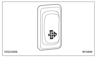
Fig. 7.5, Request/Inhibit Regen Switch
