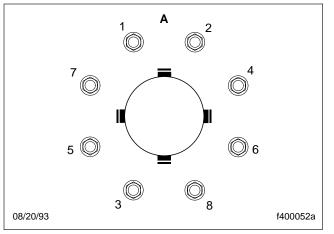
Fig. 11.8, Tightening Pattern, 8-Hole Wheels
