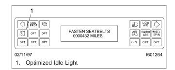
Fig. 2.21, Optimized Idle Light Location
