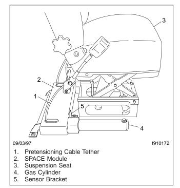
Fig. 5.12, SPACE System Components
