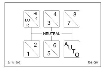
Fig. 8.14, Top 2 and Lightning Shift Patterns (with cruise control on)
