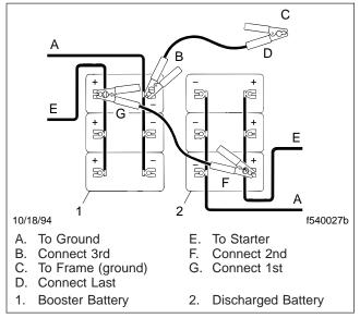
Fig. 13.3, Jumper Connections
