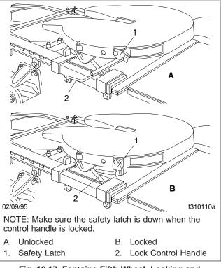
Fig. 10.17, Fontaine Fifth Wheel, Locking and Unlocking
