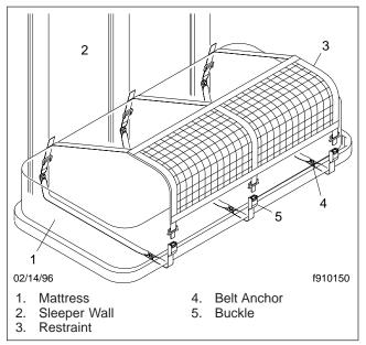
Fig. 5.11, Bunk Restraint
