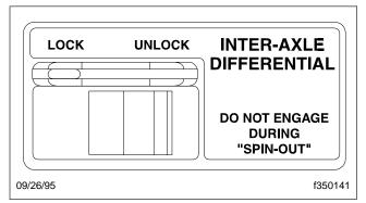
Fig. 9.2, Interaxle Differential Control
