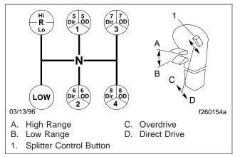
Fig. 8.17, Meritor 13-Speed Transmission Shift Pattern
