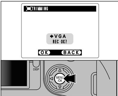
Check the size of the saved image and press the "MENU/OK" button. The trimmed image is saved as a separate file.
