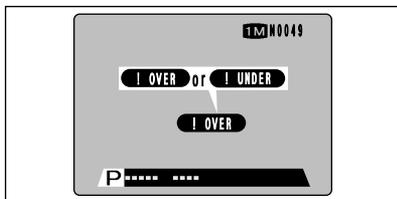
If " ! OVER " or " ! UNDER " is displayed, the white balance was not measured at the correct exposure. Reset the white balance.
