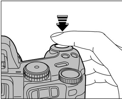
When the camera is in sleep mode, pressing the shutter button down halfway wakes the camera up so that it is ready to take pictures. This is a useful feature as it allows you to take pictures more quickly than switching the camera off and then on again.
