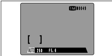
The AF frame is displayed in the location to which the target point was moved.
