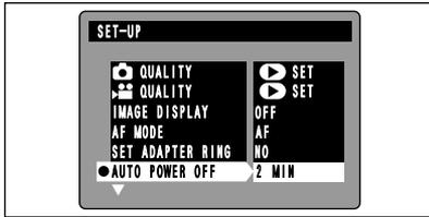
When this function is enabled, the screen temporarily switches off (sleeps) to save power if the camera is not used for approx. 30 seconds. If the camera remains unused for an additional interval (2 minutes or 5 minutes), it is automatically switched off. Use this function when you want to get the maximum possible running time from your batteries.
