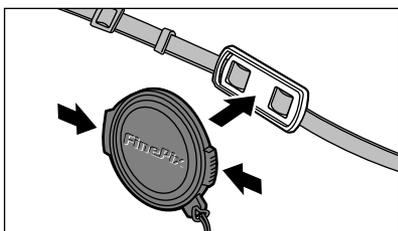
To ensure that the lens cap does not appear in your shot when you take a picture, attach it to the lens cap holder.
