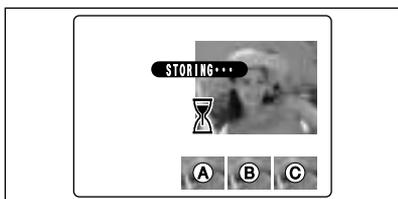
This mode automatically shoots 3 continuous frames that bracket the selected setting so that one image is correctly exposed (A), one is overexposed (B) and one is underexposed (C). The settings (exposure range) can be changed in the photography menu.
