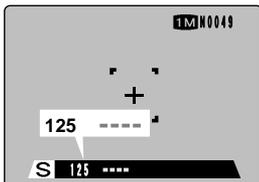
When the brightness of the subject is outside the camera's brightness metering range, “----” is displayed as the shutter speed setting. When this occurs, press the shutter button down halfway to measure the light level again and display a value.
