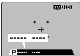
When the brightness of the subject is outside the camera's brightness metering range, "-----" is displayed as the shutter speed and aperture setting on the screen.
