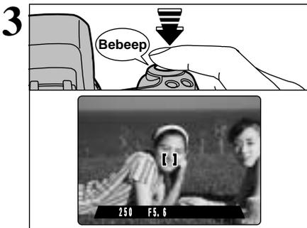
Keep holding the shutter button down halfway (AF/AE lock). Check that the AF frame shrinks and that the shutter speed and aperture settings are displayed (the indicator lamp (green) changes from blinking to lit).
