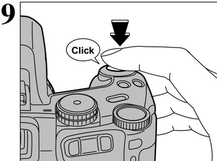
When you keep the shutter button pressed down halfway and then press it down further (pressed fully), the camera makes a soft clicking sound and takes the picture.
