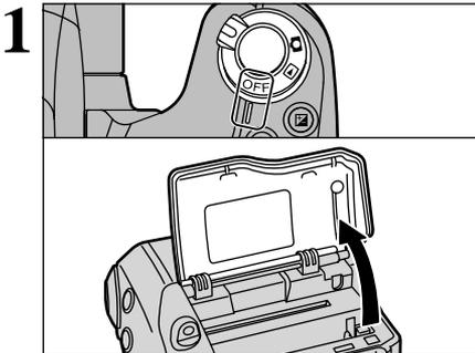
Set the Power switch to "OFF", check that the indicator lamp is off and then open the slot cover.
