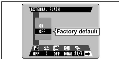
Select "ON" in this setting when you are using an external flash unit. Synchronized shutter speeds up to 1/1000 sec. can be used.
