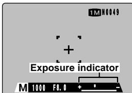
Use the exposure indicator on the screen as a guide when setting the exposure.
