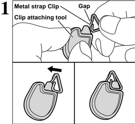
Checking that the metal strap clip is facing the right way, slide the clip fully into the clip attaching tool and open up the gap in the strap clip.
