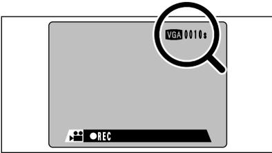
A counter displayed in the top-right corner of the screen during shooting shows the remaining time.
