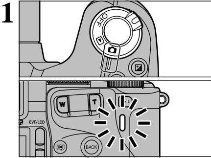
To switch the camera on, set the Power switch to “**ON**” or “**▶**”. When you switch the camera on, the indicator lamp lights green.
