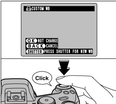
Under the light source you want to set the white balance for, hold a piece of white paper so that it fills the screen and press the shutter button to set the white balance.
