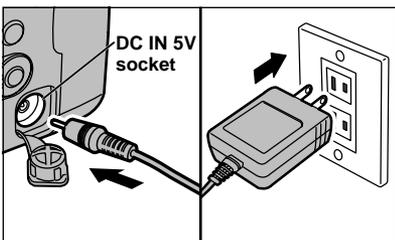
Check that the camera is switched off. Open the terminal cover and plug the AC power adapter connector into the “DC IN 5V” socket. Then plug the AC power adapter into a power outlet.
