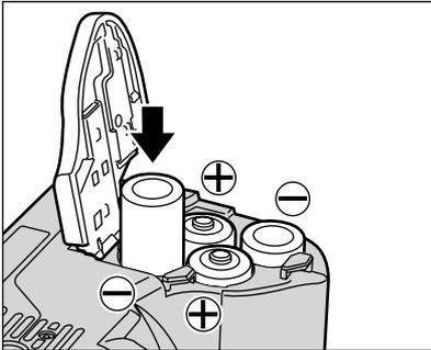
Insert the batteries correctly as indicated by the polarity icons.
