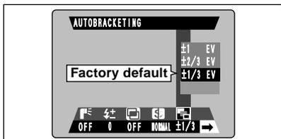
Use this feature to photograph the same image with different exposure settings. Auto bracketing automatically shoots 3 consecutive frames, one of which is correctly exposed while the remaining two are underexposed and overexposed respectively by a set amount.
