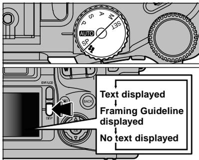
This function can be selected in the “**AUTO** • SP • P • S • A and M” photography modes. The screen display changes each time you press the “**DISP**” button. Press the “**DISP**” button to display the framing guideline.
