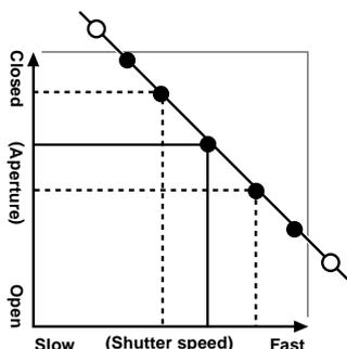
The graph at left shows the way the aperture and shutter speed settings can be changed while maintaining the same exposure level.
