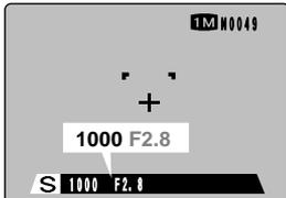
In scenes that are extremely underexposed, the aperture setting (F2.8) is displayed in red. When this occurs, select a slower shutter speed (down to 3 sec.).
