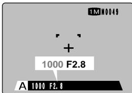
In scenes that are extremely overexposed, the shutter speed (1/1000 sec.) is displayed in red. When this occurs, select a larger aperture (up to F11.).
