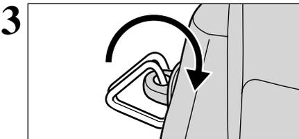
Turn the metal strap clip around once until it clicks closed and is fully threaded onto the strap mount.
