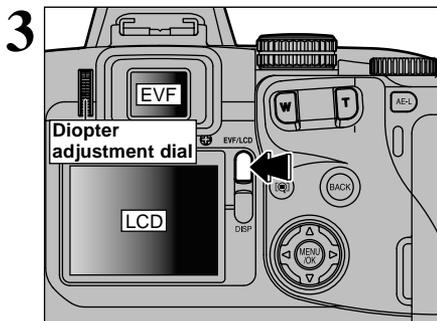
Each time you press the “EVF/LCD” button, display switches between the viewfinder (EVF) and the monitor (LCD). If the AF frame in the viewfinder (EVF) is difficult to see, adjust the viewfinder using the diopter adjustment dial.
