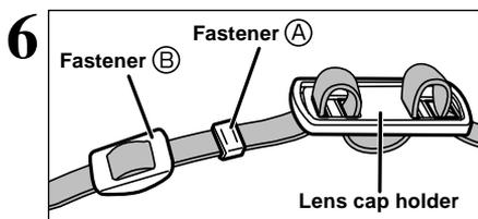
Remove fasteners **A** and **B** from only one side of the shoulder strap. Then pass the shoulder strap through the lens cap holder and then back through fasteners **A** and **B**.
