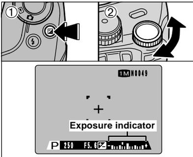
To select the Exposure Compensation setting, hold down the “**Fn**” button ① and turn the Command dial ②. The “**Fn**” symbol also turns yellow while exposure compensation is being set and then turns blue after setting is completed.
