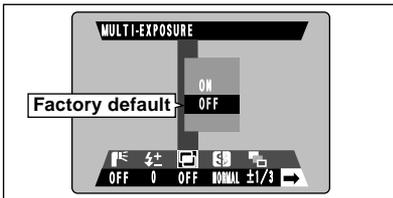
Multiple-exposure provides a way of overlaying photographed images on top of each other to give a final image that cannot be obtained through normal photography.
