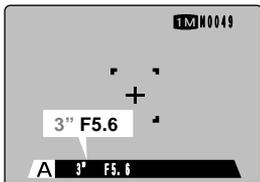
In scenes that are extremely underexposed, the shutter speed (3 sec.) is displayed in red. When this occurs, select a smaller aperture (down to F2.8.).
