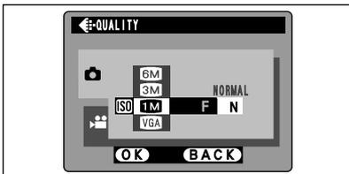
If you hold down the “**SHIFT**” button and press the “**MENU/OK**” button, the menu is displayed but the **QUALITY** setting cannot be changed from “**1M**” and **NORMAL**.
