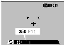
In scenes that are extremely overexposed, the aperture setting (F11) is displayed in red. When this occurs, select a faster shutter speed (up to 1/1000 sec.).
