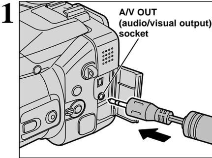
Switch off the camera and TV. Open the terminal cover and plug the A/V cable (provided with the camera) into the “A/V OUT” (audio/video output) socket.
