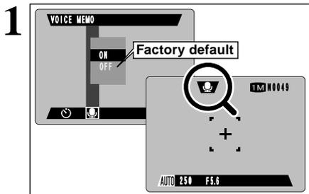
If you set voice memo to ON, “” appears on the screen. This function allows you to add a voice memo up to 30 seconds long to an image immediately after you take the picture. Note that this function cannot be used with continuous shooting.
