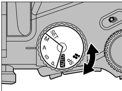
The mode can be set to "P • S • A" (⇒P.35, 36, 37) or "M" (⇒P.38), but the use of "A" or "M" is recommended.
