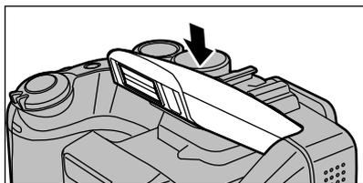
Pressing the flash down switches the camera to Suppressed Flash mode.
