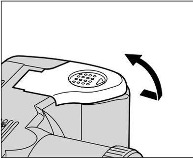
Slide the battery cover out and lift it open.
