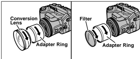
Mount the Adapter Ring, Conversion Lens and commercially available filters by screwing them on in the direction of the arrow.
