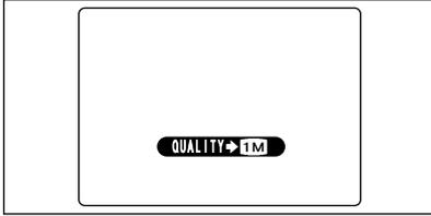
This mode allows you to take up to 40 continuous shots (at intervals as short as 0.6 seconds). In Long-period Continuous Shooting with 1280 × 960-pixel mode, the number of recorded pixels is automatically set to "1M" (1280 × 960 pixels). You can select NORMAL or FINE as the quality setting (⇒P.69).
