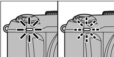
The self-timer lamp lights and then starts flashing until the picture is taken.
