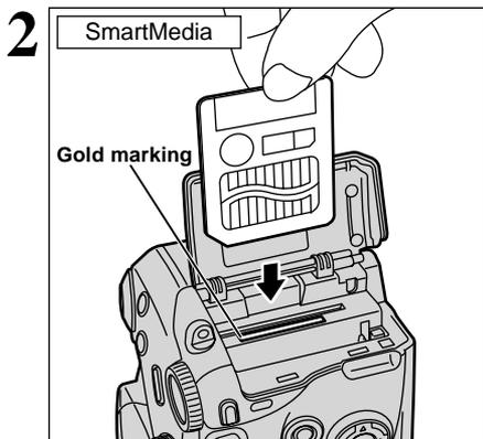
Push the SmartMedia firmly all the way into the SmartMedia slot.
