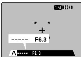
When the brightness of the subject is outside the camera's brightness metering range, "----" is displayed as the aperture setting. When this occurs, press the shutter button down halfway to measure the light level again and display a value.
