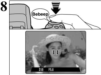
When you press the shutter button down halfway, the camera emits a short double-beep and focuses on your subject. At that point, the AF frame on the screen becomes smaller and the camera sets the shutter speed and aperture.
