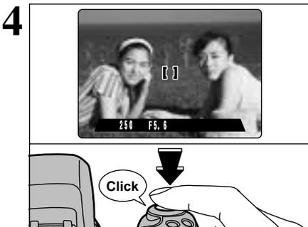
Continue to hold the shutter button down halfway (AF/AE lock). Move the camera back to the original image and then fully press down on the shutter button.
