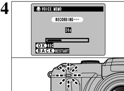
The remaining recording time is displayed during recording and the self-timer lamp flashes.
