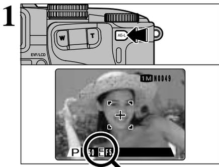
Use this function when you want to take pictures with the exposure fixed for a particular subject. Frame the shot so that the subject occupies most of the center of the screen and then press the “AE-L” button.
