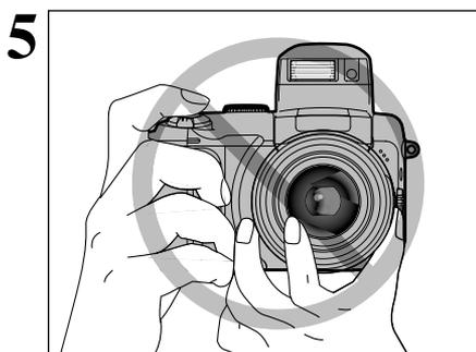
Make sure that the strap or your fingers are not covering the lens, AF sensor, flash control sensor or microphone. The shot will not be taken successfully if any of these camera components is obscured by your fingers or by the strap.
