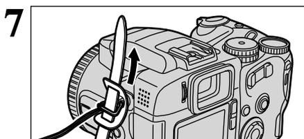
Thread the strap through the protective cover and metal strap clip.
