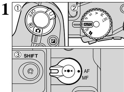
1 Set the Power switch ① to "📷" and the mode dial ② to "AUTO". Then set the focus mode selector switch ③ to "AF".
