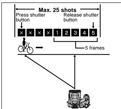
This mode allows you to release the shutter up to 25 times (at intervals as short as 0.2 seconds) and record the last 5 frames. If you take your finger off the shutter button before 25 shots have been taken, the camera records the final 5 frames shot before you released the shutter button.
