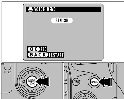
After 30 seconds of recording, "FINISH" appears on the screen.
