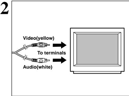
Plug the other end of the cable into the video input socket on the TV. Then switch the camera and TV on and take pictures or play back images as you would normally.
