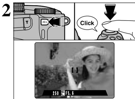
With the “AE-L” button held down, press the shutter button down halfway to focus the shot and then compose the shot again.
