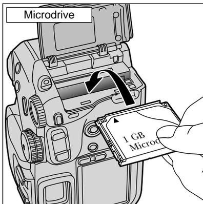
Push the Microdrive firmly all the way into the Microdrive slot.
