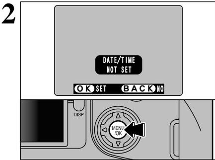
When you first switch the camera on, the date is cleared. Press the “**MENU/OK**” button to set the date and time.
