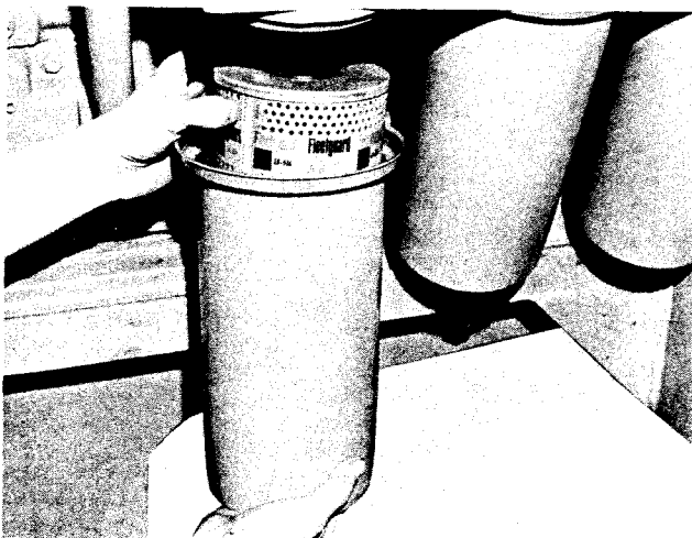
Fig. 2-13 (V40737) Removing lubricating oil filter element(s)
