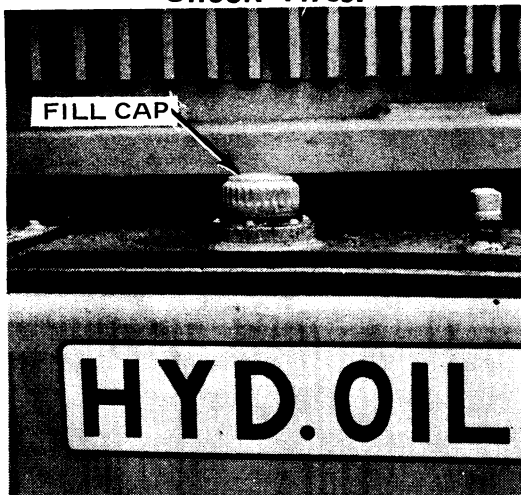
Check Reservoir Level.
