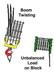
When reconfiguring the reeving on the load block, the parts of line need to be evenly spaced on both sides of the hook to prevent the block from tilting when picking up a load. Flange damage to the sheaves can result from operating like this.
