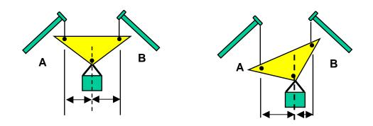
When the load is lifted by a beam and all the load attachment points <u>ARE NOT</u> in a straight line with the crane's attachment points, one crane may become overloaded. If crane A lowers its end and the beam rotates to the left, the loading on crane B increases because the horizontal distance from the load's center of gravity to crane B has decreased.
