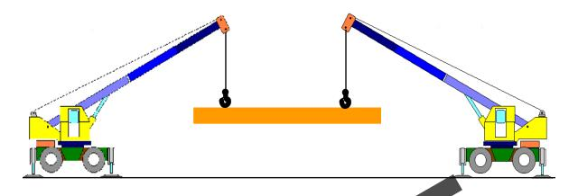
There are occasions when it may be necessary to lift a load with two cranes. These lifts should be done with experienced crane operators and under the supervision of an experienced signal person to coordinate the lift. Each crane must be set up properly, and the load weight imposed on each crane must be accurately determined.
