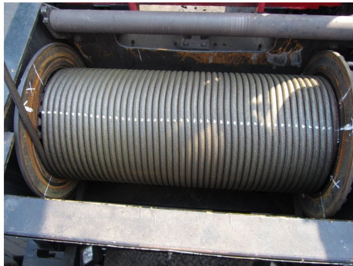
The rope is loaded with 10% SWL and marked under load
