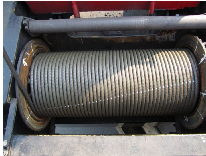
The rope is unloaded - illustrating the affects of elongation.
