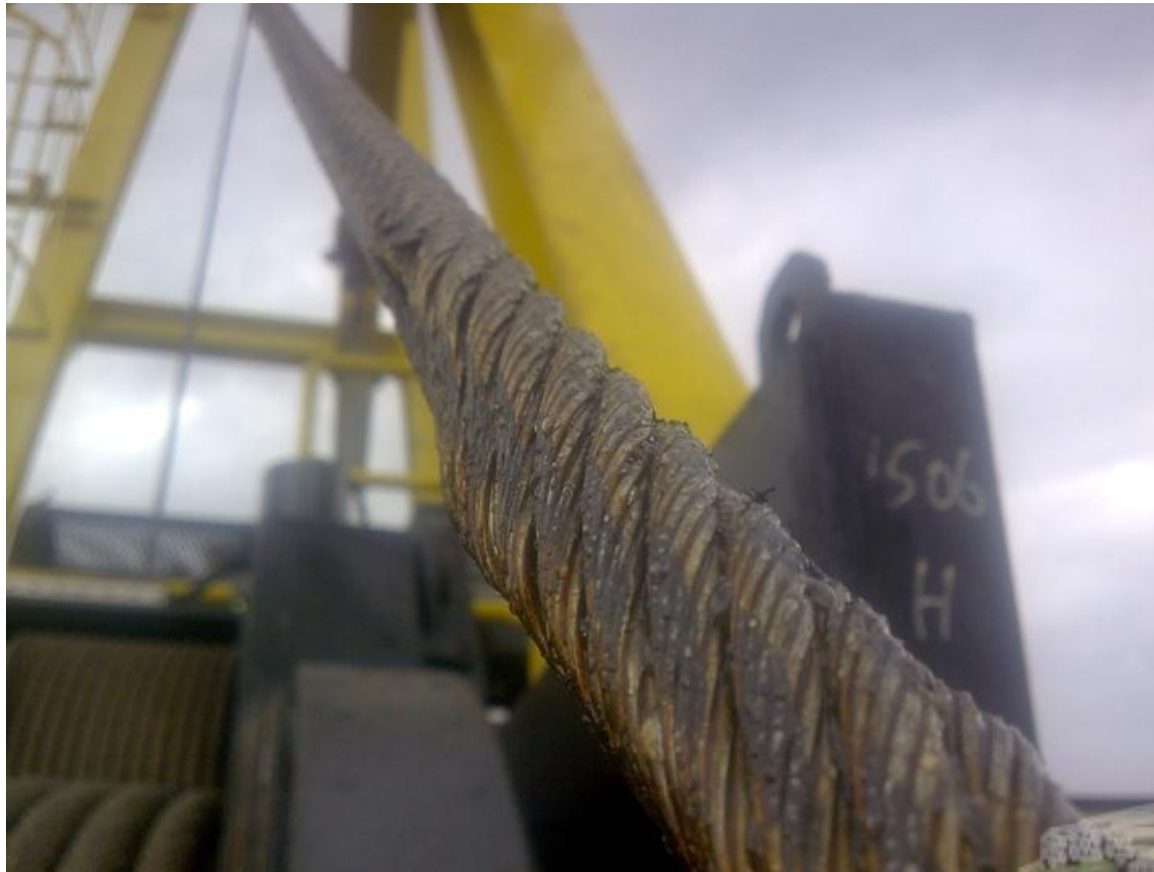
Damage to a boom hoist rope due to insufficient rope tension
