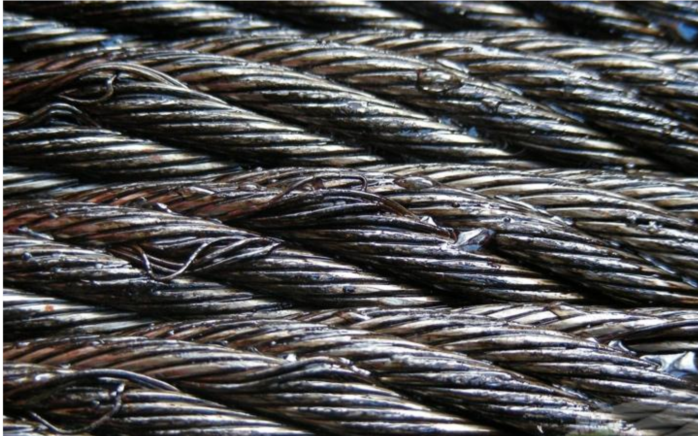
Damage to a boom hoist rope due to insufficient rope tension
