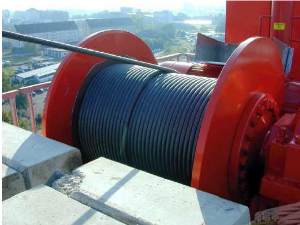
Typical multi-layer drum (on a tower crane)
