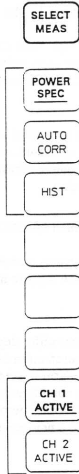
Figure 6-8. SELECT MEAS Menu Diagram: Time Capture Mode
