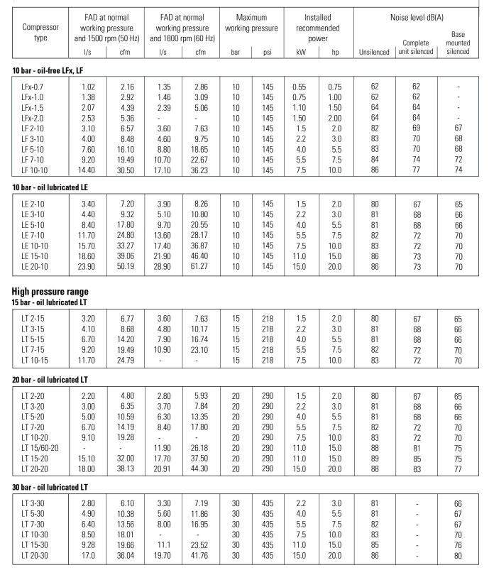
LE / LT / LF 2-10 with integrated refrigerant dryers and filter package.
