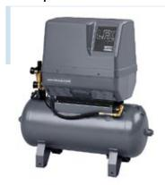
Power box mounted on an internally epoxy painted 50 or 100 litre air receiver, including regulation, safety valve, pressure regulator, outlet valve and pressure gauge. The complete silenced compressed air installation. For 60 Hz units, receivers are ASME approved as standard. For 50 Hz units, receivers are CE/AS1210 (only 50 I) approved.
