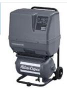
Power box mounted on an internally epoxy painted 20 litre air receiver (CE/AS1210 for 50 Hz, ASME for 60 Hz), including regulation, safety valve, pressure regulator, regulated outlet valve, pressure gauges and trolley frame. Overload protection is included for 3-phase units.
