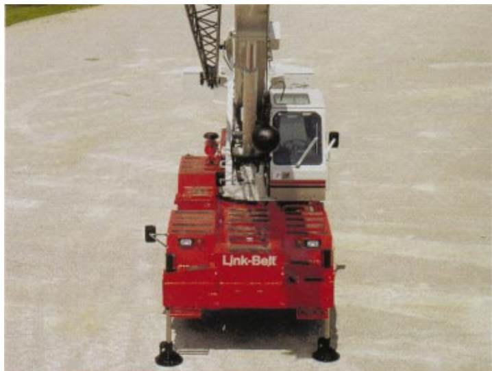
Fully Retracted Outriggers – 7' 4-3/4" (2.25 m) spread
