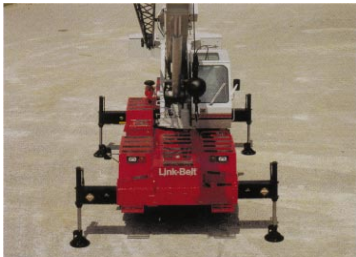
Intermediate Extended Outriggers – 12' 11-3/4" (3.96 m) spread
