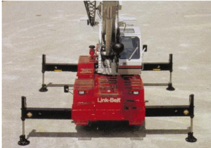
Fully Extended Outriggers – 18' 6-3/4" (5.66 m) spread
