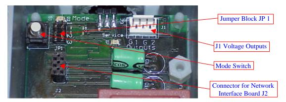
Jumpers 1-3 on jumper block JP1 take priority over the network Humidity Setpoint, nciRHSetpoint. The jumpers are used as follows:
