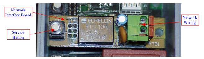
The Network Interface Module can actually be plugged into a unit to configure it and then removed before the unit is put into service. The Model 2500 will retain the configuration parameters even after the Network Interface Module is removed. The interface also includes the Service switch used to install onto a LonWorks network.
