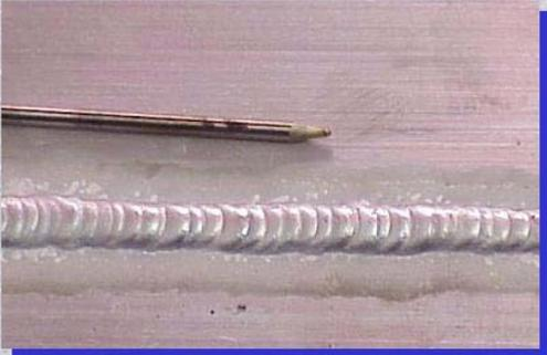
A close-up photograph of a steel rebar with a weld. The weld is characterized by a distinct, regular, repeating pattern of ripples along its length, which is typical for a 60 Hz AC welding process.
