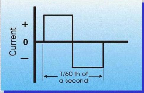
The graph shows a square wave current signal. The vertical axis is labeled 'Current' with '+' above the zero line and '-' below. The horizontal axis represents time. A double-headed arrow below the axis indicates a duration of  $1/60$  th of a second, corresponding to one full cycle of the 60 Hz signal.
