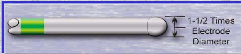
Use a balled, pure tungsten electrode for:
