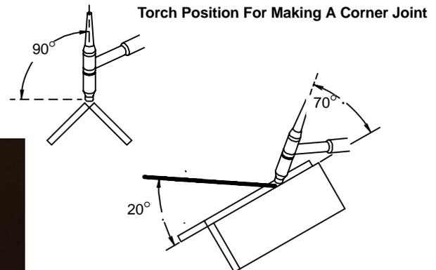
**Torch Position For Making A Corner Joint**
