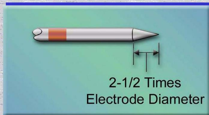
Use a sharpened, tungsten alloy electrode for:
