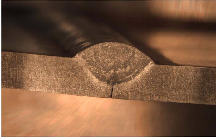
The arc shaping capabilities of our inverter products help produce superior weldments as shown in the photo. This weld was made in a controlled environment. Your results may vary due to things such as operator skill, type of material and material thickness, shielding gas, atmospheric conditions, and joint preparation, etc.
