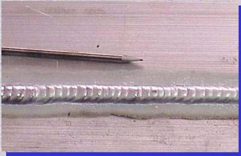
A close-up photograph of a steel rebar with a weld. The weld surface is significantly smoother and more uniform than the 60 Hz weld, due to the higher frequency of the AC power source.
