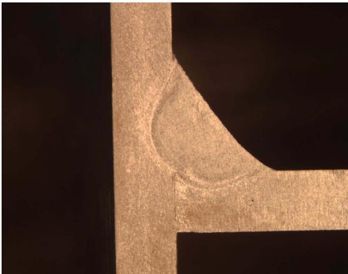
The arc shaping capabilities of our inverter products help produce superior weldments as shown in the photo. This weld was made in a controlled environment. Your results may vary due to things such as operator skill, type of material and material thickness, shielding gas, atmospheric conditions, and joint preparation, etc.
