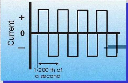
The graph shows a square wave current signal with a higher frequency than the 60 Hz signal. The vertical axis is labeled 'Current' with '+' above the zero line and '-' below. The horizontal axis represents time. A double-headed arrow below the axis indicates a duration of  $1/200$  th of a second, corresponding to one full cycle of the 200 Hz signal.
