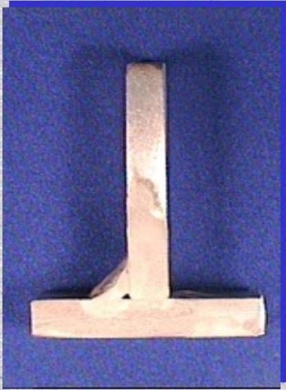
A photograph of a T-joint weld on a metal plate. The weld is a smooth, continuous line, indicating a high-quality weld achieved with a 60 Hz AC power source.
