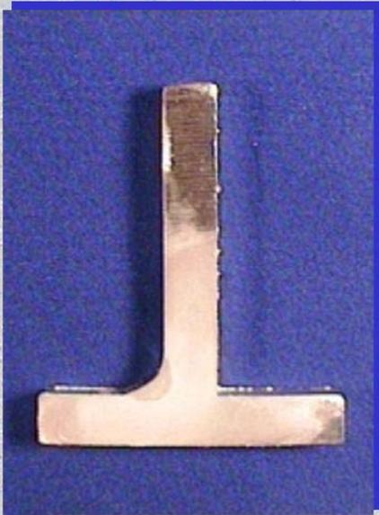
A photograph of a T-joint weld on a metal plate. The weld is very smooth and uniform, demonstrating the benefits of a 200 Hz AC power source for welding.
