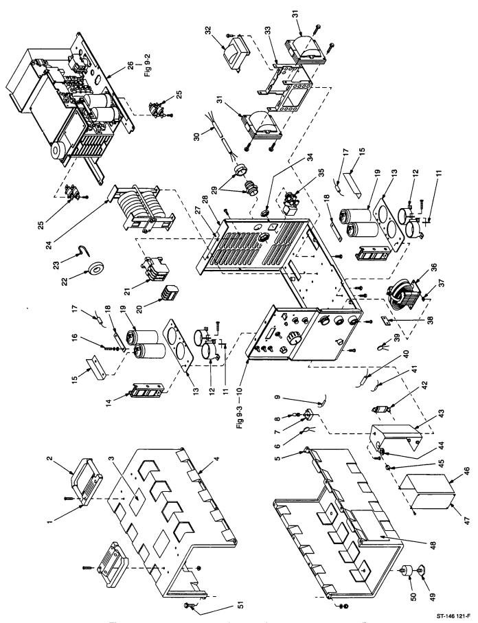
Figure 9-1. Main Assembly (208-230/460V Model Illustrated)
