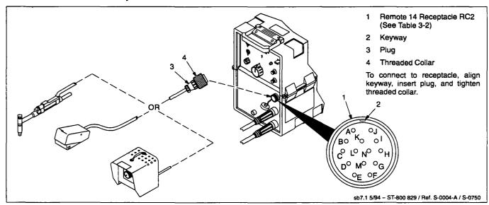
Figure 3-6. Remote 14 Connections
