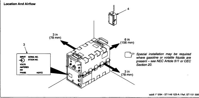
Figure 3-2. Location And Movement Of Welding Power Source
