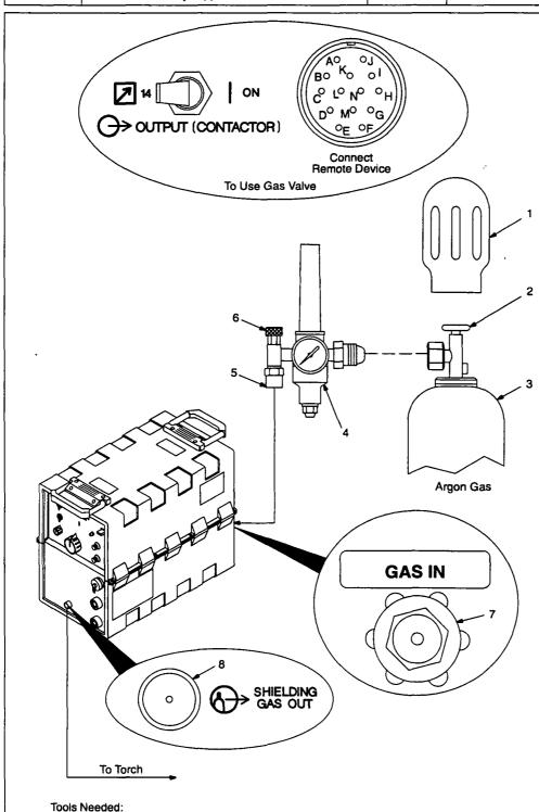
Obtain gas cylinder and chain to running gear, wall, or other stationary support so cylinder cannot fall and break off valve.
