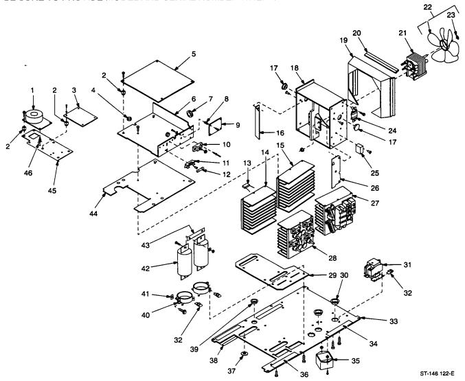
Figure 9-2. Chassis, Mid (208-230/460V Model Illustrated)
