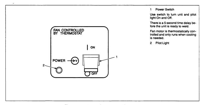
Figure 4-11. Power Switch And Pilot Light
