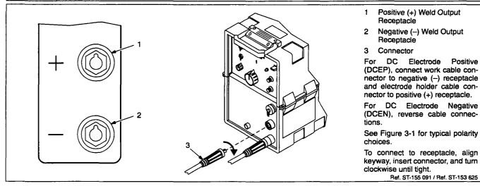
Figure 3-5. Connecting To Weld Output Receptacles
