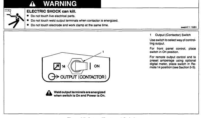
Figure 4-7. Output (Contactor) Switch
