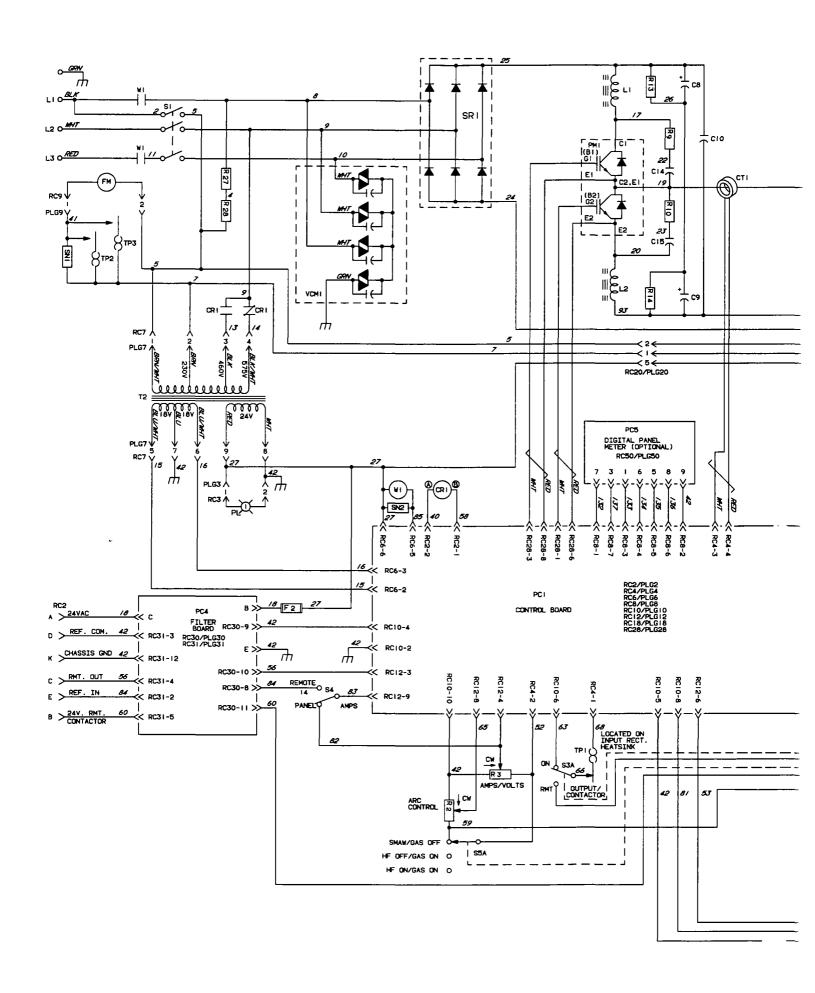
Figure 6-2. Circuit Diagram For 460/575 Volt Models
