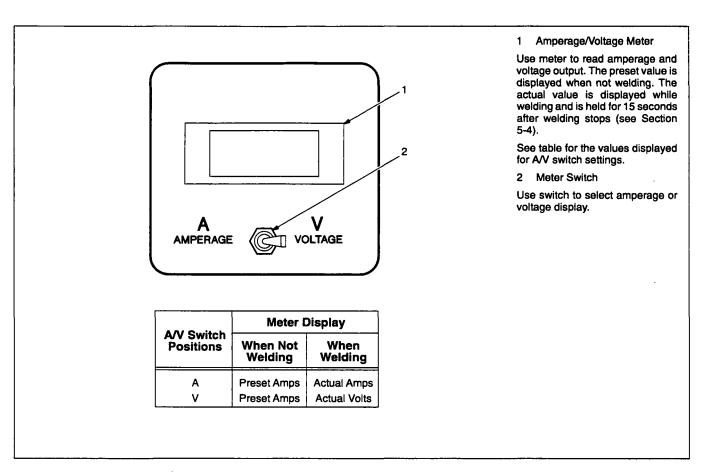
Figure 4-10. Amperage/Voltage Meter And Switch (Optional)
