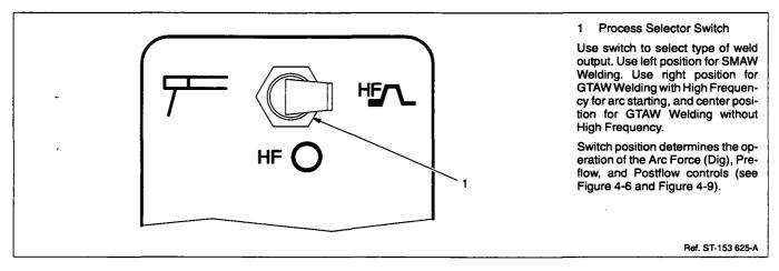
Figure 4-4. Process Selector Switch
