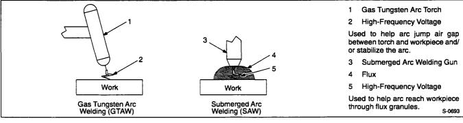
Figure 7-1. Welding Processes Requiring High Frequency
