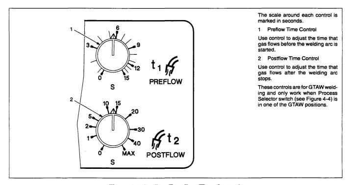
Figure 4-9. Preflow/Postflow Time Controls
