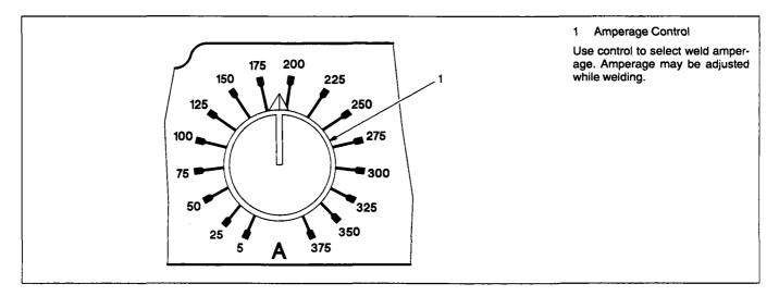
Figure 4-5. Amperage Control
