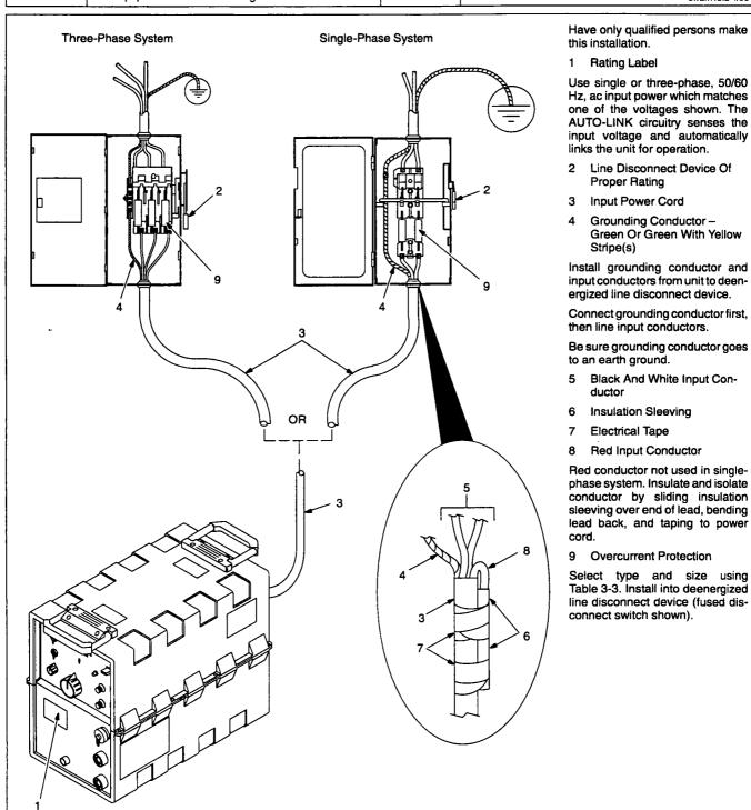
Figure 3-8. Input Power Connections
