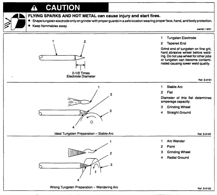
Figure 8-2. Preparing Tungsten For DC Electrode Negative (DCEN) Welding
