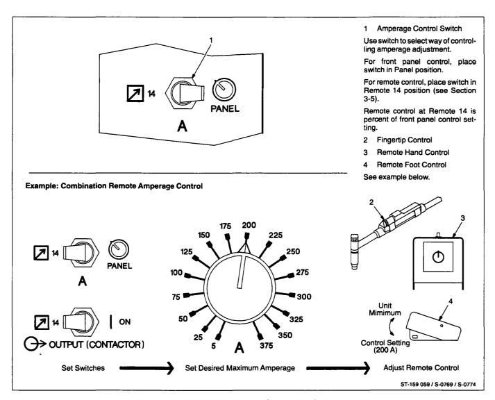
Figure 4-8. Amperage Control Switch
