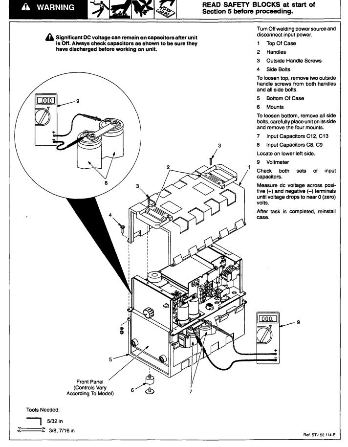
Figure 5-2. Removing Case And Measuring Input Capacitor Voltage
