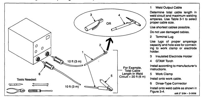
Figure 3-3. Selecting And Preparing Weld Output Cables
