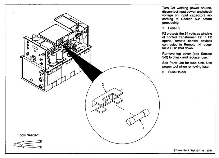
Figure 5-4. Overload Protection
