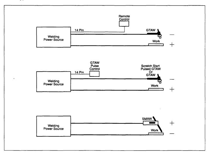
Figure 3-1. Typical Process Connections
