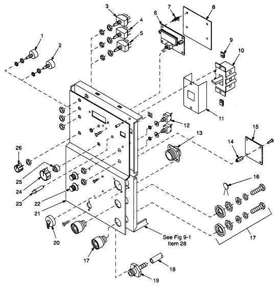
Figure 9-3. Panel, Front w/Components
