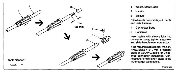
Figure 3-4. Dinse-Type Connector Assembly
