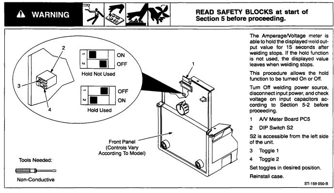
Figure 5-5. Changing Amperage/Voltage Meter Hold Function
