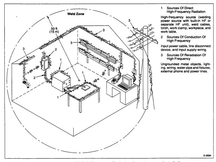
Figure 7-2. Sources Of High-Frequency Radiation From Incorrect Installation
