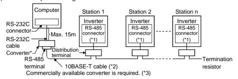
Use the connectors, cables and converter which are available on the market. Introduced products (as of June, 2000)
