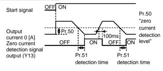
To prevent this, the output current "zero" signal can be output from the inverter to close the mechanical brake when the output current has fallen to "zero".
