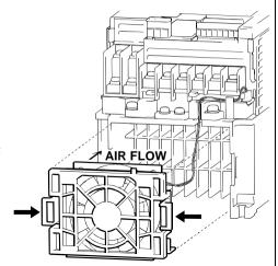
4) Remove the cooling fan and cooling fan cover.The cooling fan is secured by the fixing catches.Disengaging the fixing catches removes the cooling fan and cooling fan cover.
