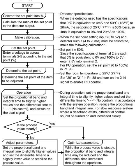
\*When calibration → Use Pr. 38 and calibration parameters C2 to C4 (terminal 2) is required and Pr. 39 and calibration parameters C5 to C7 (terminal 4) to calibrate the detector output and set point setting input.
