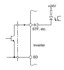
External signal input using transistor
