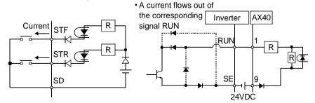
Connecting a positive external power supply for transistor output to terminal PC prevents a malfunction caused by a undesirable current. (Do not connect terminal SD of the inverter with terminal 0V of the external power supply. When using terminals PC-SD as a 24VDC power supply, do not install an external power supply in parallel with the inverter. Doing so may cause a malfunction in the inverter due to a undesirable current.)
