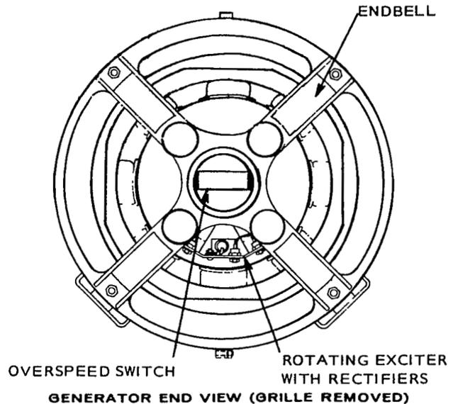
FIGURE 22. ROTATING RECTIFIER ASSEMBLY
