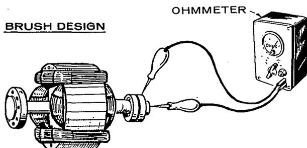
CONTACT ONE PROD TO EACH OF THE SLIP RINGS AND THE OTHER PROD TO THE ROTOR SHAFT. IF ROTOR IS GOOD THERE SHOULD BE NO READING ON OHMMETER.
