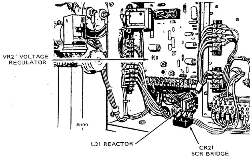
FIGURE 23. SCR BRIDGE AND REACTOR LOCATION
