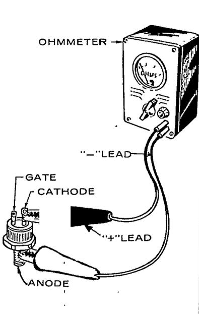
FIGURE 9. TESTING SCR's
