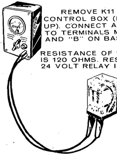
REMOVE K11 OR K12 FROM CONTROL BOX (PULL STRAIGHT UP). CONNECT AN OHMMETER TO TERMINALS MARKED "A" AND "B" ON BASE OF RELAY.
