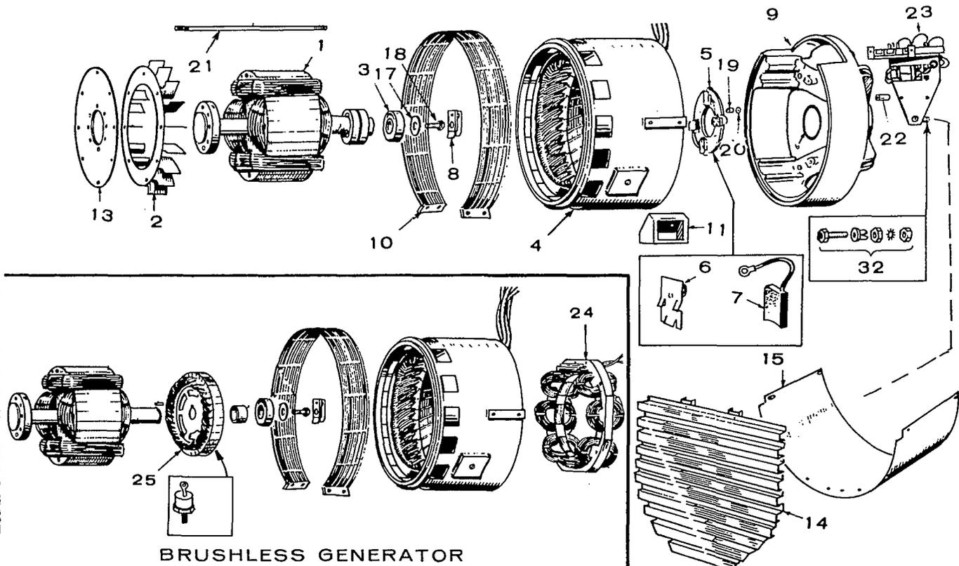
FIGURE 20. GENERATOR DISASSEMBLY
