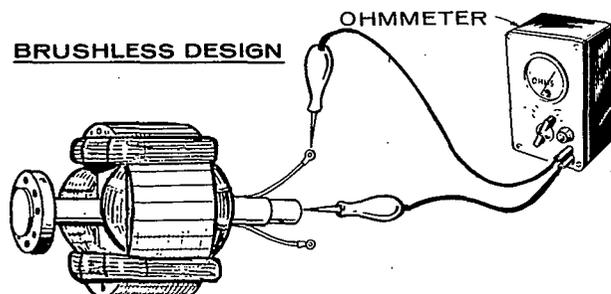
CONTACT ONE PROD TO EACH OF THE FIELD LEADS AND THE OTHER PROD TO THE ROTOR SHAFT. IF ROTOR IS GOOD THERE SHOULD BE NO READING ON OHMMETER.
