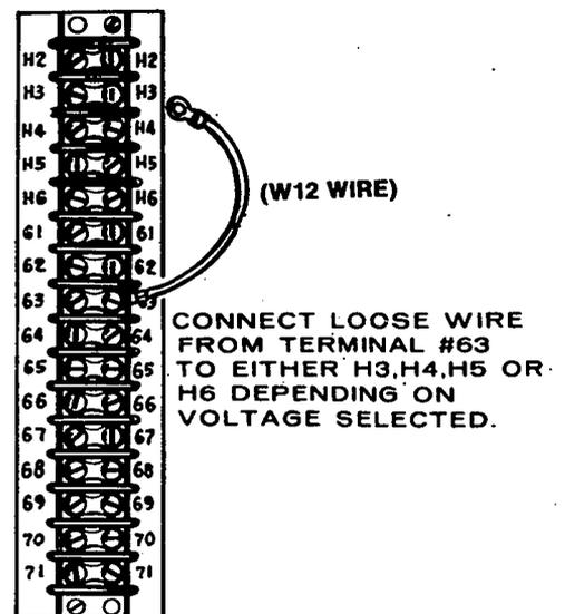
FIGURE 17. CONNECTING LEAD FROM TERMINAL 63
