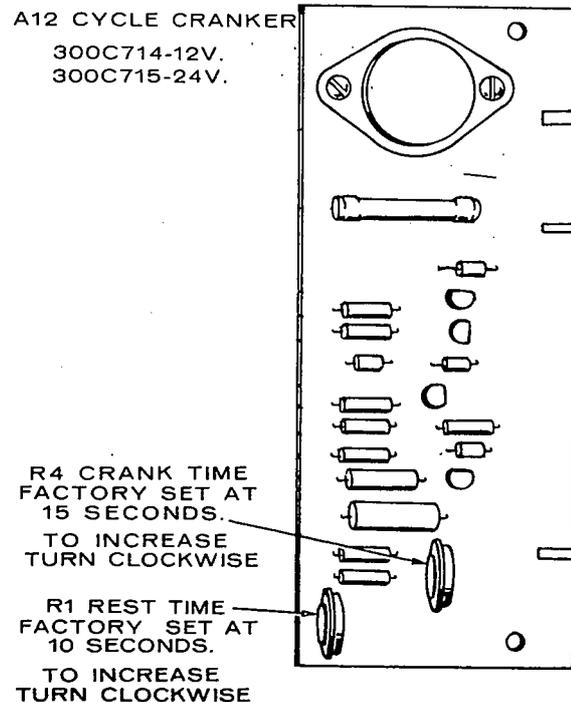
FIGURE 33. OPTIONAL CYCLE CRANKER ADJUSTMENTS
