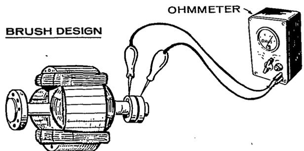
CONTACT ONE PROD TO ONE SLIP RING AND THE OTHER PROD TO THE SECOND SLIP RING.
