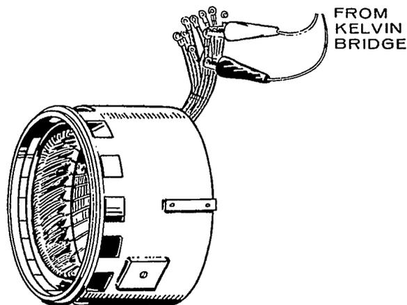
FIGURE 14. TESTING STATOR WINDINGS
