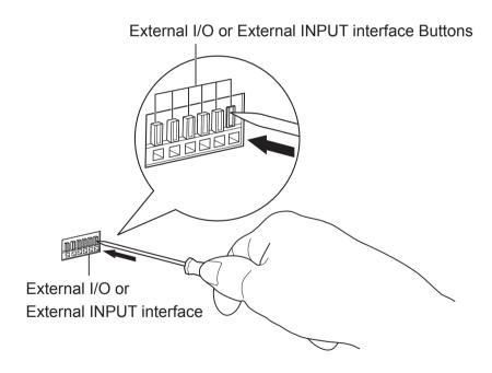
A 6-terminal interface is shown here. The number of interface terminals varies by camera model.
