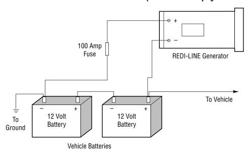
If the load requirement is not heavy (intermittent hand tool use or light loads for a long period of time) the vehicle battery and charging system should handle both the vehicle and additional generator demand.
