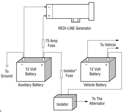
If the load requirements are heavy (constant use of hand tools or large loads) install one or more auxiliary deep cycle batteries. The auxiliary battery should be isolated from the vehicle battery using a battery isolator. The battery isolator is a one way path so both batteries are charged by the vehicle but one battery cannot discharge the other. This will ensure the vehicle battery is always charged and you will be able to start your vehicle.
