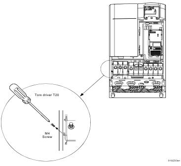
Figure 5. Disconnecting Y Capacitor in SED2 Frame Size D and E.
