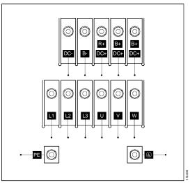
Figure 14. Power and Motor Terminal Layout for SED2 (IP20) Frame Size F with Built-in EMC Filter.
