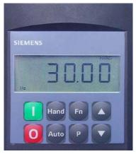
Figure 20. Basic Operator Panel.
