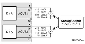
Figure 30. SED2 Analog Outputs 1 and 2.
