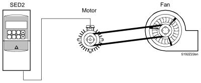
Figure 32. Belt Failure Detection without Sensor (P2181).
