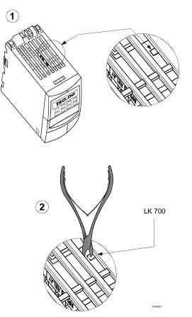
Figure 3. Disconnecting Y Capacitor in SED2 Frame Size A.
