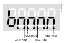
Figure 27. Allocation of Each Input to a Display Segment using Parameter r0722.
