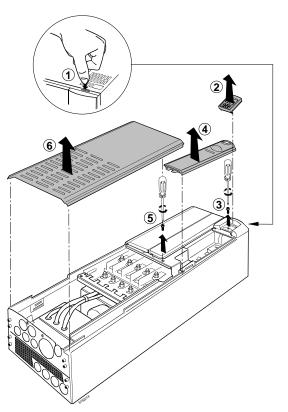
Figure 10. Access to Connection Terminals for SED2 Frame Size F.
