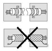
Figure 2. Use Grounding Clamps to Bond the Shield.
