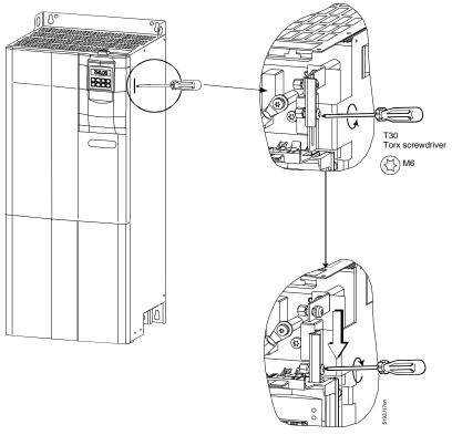
Figure 6. Disconnecting Y Capacitor in SED2 Frame Size F.
