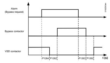
Figure 11. Bypass Timing Diagram.
