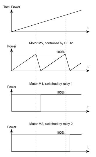
Figure 37. Diagram From Motor Staging.
