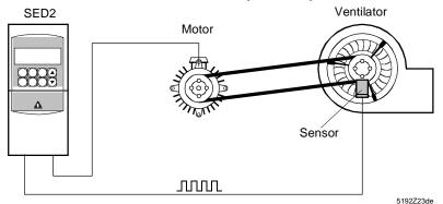
Figure 34. Belt Failure Detection with Sensor (P0400).
