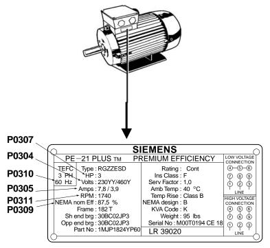
Figure 22. Motor Nameplate Data for Commissioning Parameters.
