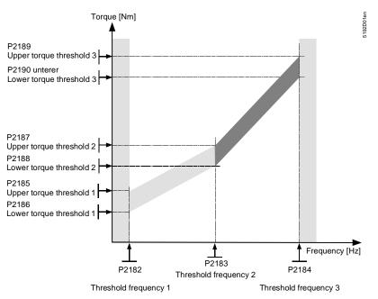
Figure 33. Frequency/Torque Curve.
