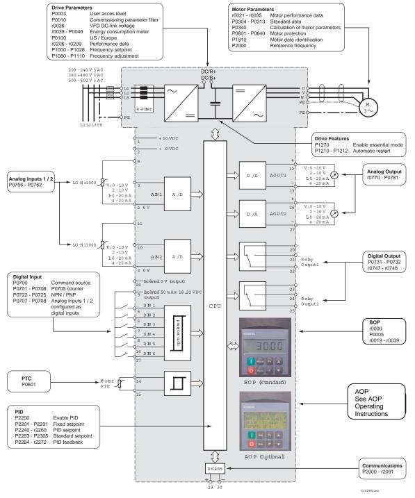
Figure 24. Block Diagram of SED2 Parameters.
