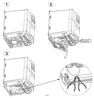
Figure 4. Disconnecting Y Capacitor in SED2 Frame Size B and C.
