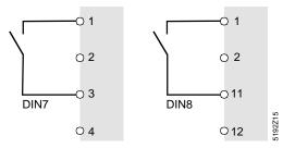
Figure 26. Connection of Analog Inputs 1 and 2 as Digital Inputs 7 and 8.
