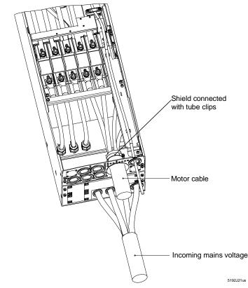
Figure 5. Cable Routing for SED2 (IP20) Frame Size D through F with EMC Filter.
