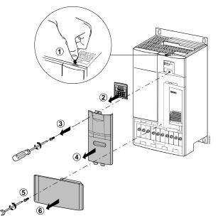
Figure 9. Access to Connection Terminals for SED2 Frame Size D and E.
