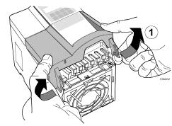
Figure 8. Access to Connection Terminals for SED2 Frame Size B and C.
