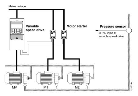
MV: Motor, speed-controlled by SED2.
