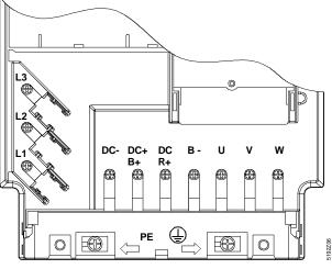
Figure 12. Power and Motor Terminal Layout for SED2 Frame Size B and C.
