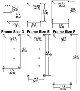
**Mounting Clearance:** Leave 4 inches (102 mm) of space at top and bottom for equipment access. (If fitted with a protective shield, allow 12 inches [305 mm] of space between the sides of each VFD to allow for sufficient heat dissipation.)
