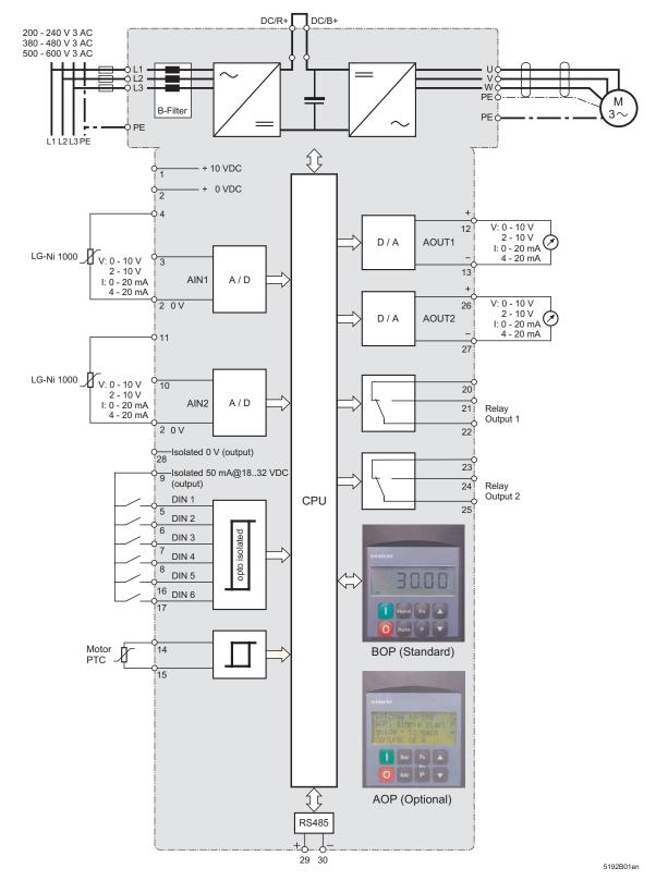
Figure 18. SED2 Control Terminal Block Diagram.
