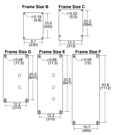
Figure 2. Mounting Dimensions of SED2 (IP54, NEMA Type 12). Dimensions in Inches (Millimeters).
