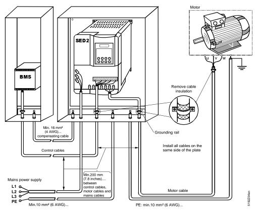
Figure 3. Routing Control, Mains, and Motor Cables.
