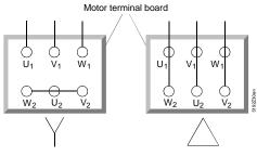
Figure 16. Delta and Star (Wye, Y) Motor Connections.
