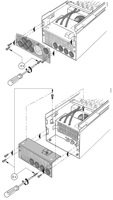
SED2 drives (frame sizes D, E, and F) include a built-in, prewired, EMC filter. Route and connect the mains power to the terminals of the filter.
