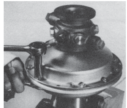
Figure 7-10 Bolting upper and lower housings together.
