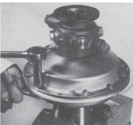
Figure 4-6 Removing housing screws and nuts.
