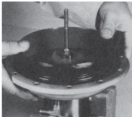
Figure 7-7 Pressing cylinder into lower housing.
