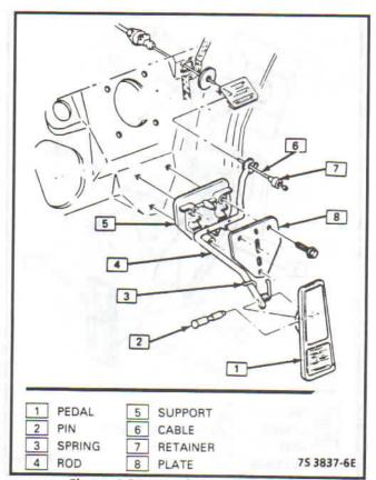
Figure 4-84 - Accelerator Pedal - RV
