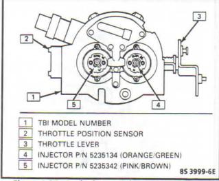
Figure 4-25 - Fuel Injector Color Code Locations TBI 220 (4.3L Engine C/K Series)
