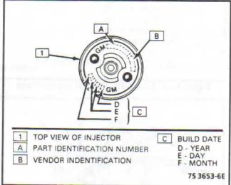
Figure 4-26 - Fuel Injector Port Number Lacation TBI 220
