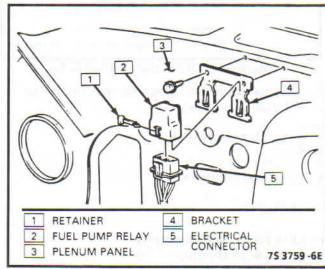
Figure 4-43 - Fuel Pump Relay (RV)
