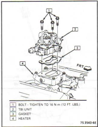
Figure 4-20 - Replacing TBI 220 Unit - 7.4L Engine
