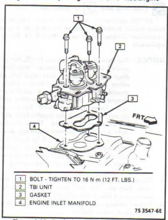
Figure 4-19 - Replacing TBI 220 Unit - 5.0L/5.7L Engine
