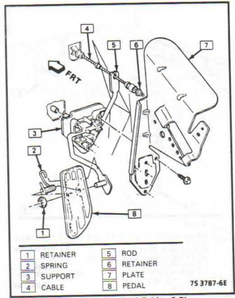
Figure 4-81 - Control Cable - 2.5L
