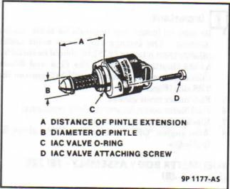
Figure 4-31 - Flange Mounted Type IAC Valve
