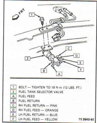
Figure 4-60 - Selector Valve - (RV)
