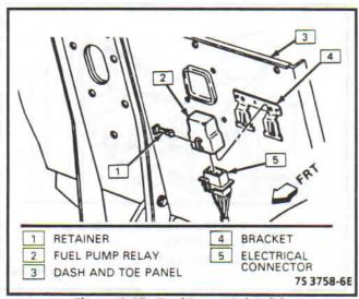
Figure 4-45 - Fuel Pump Relay (P)
