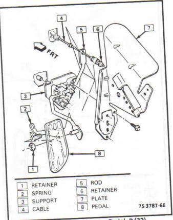
Figure 4-88 - Accelerator Pedal -P (32)
