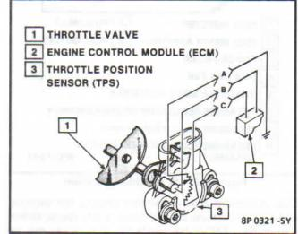
Figure 4-11 - Throttle Position Sensor (TBI 220)
