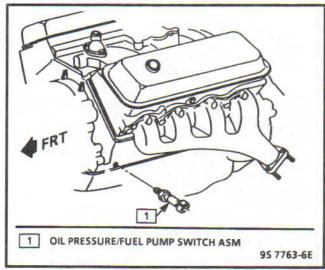
Figure 4-52 - Oil Pressure Switch (7.4)
