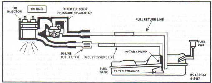
Figure 4-13 - TBI Fuel Supply System (Typical)
