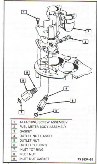
Figure 4-28 - Fuel Meter Body Assembly - TBI 220
