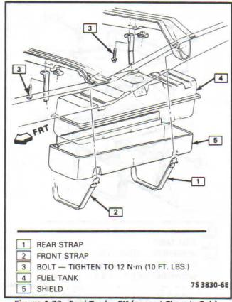
Figure 4-73 - Fuel Tank - CK (except Chassis Cab)
