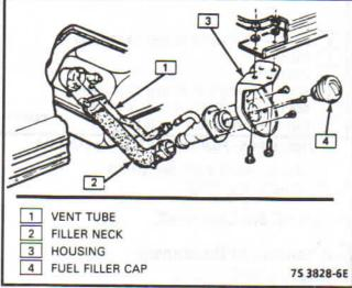
Figure 4-68 - Filler Neck - RV Chassis Cab
