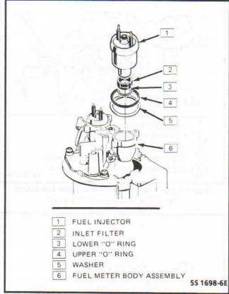
Figure 4-23 - Model TBI 220 Fuel Injector Parts
