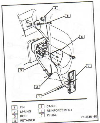
Figure 4-86 - Accelerator Pedal - G
