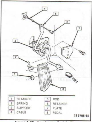
Figure 4-85 - Accelerator Pedal - CK
