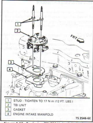
Figure 4-16 - Replacing TBI 700 Unit - 2.5L Engine
