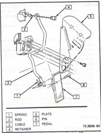
Figure 4-82 - Accelerator Pedal -ST
