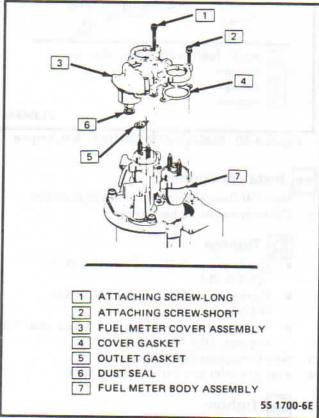
Figure 4-22 - Replacing Model 220 Fuel Meter Cover
