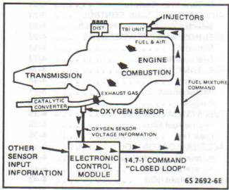
Figure 4-1 - "Closed Loop" TBI System
