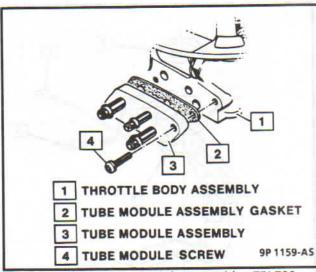
Figure 4-38 - Tube Module Assembly - TBI 700
