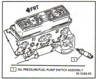
Figure 4-51 - Oil Pressure Switch (4.3 5.0, 5.7)
