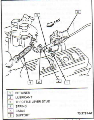
Figure 4-80 - Control Cable - 4.3L & V-8
