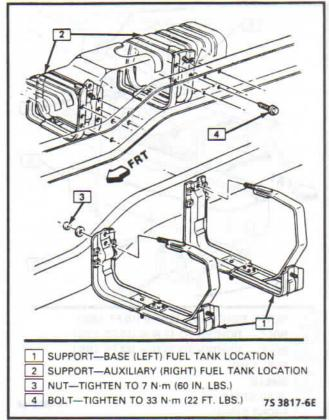
Figure 4-74 - Fuel Tank - RV Pickup
