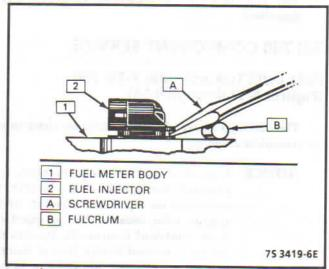
Figure 4-33 - Removing TBI 700 Fuel Injector
