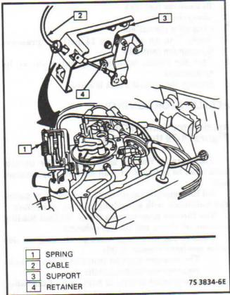
Figure 4-79 - Control Cable - 2.8L
