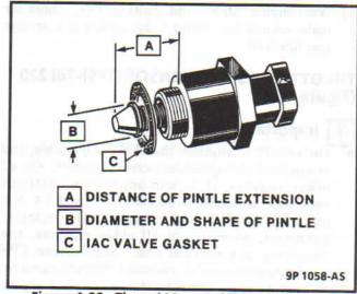
Figure 4-30 - Thread Mounted Type IAC Valve
