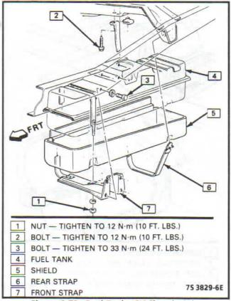
Figure 4-72 - Fuel Tank - CK Chassis Cab
