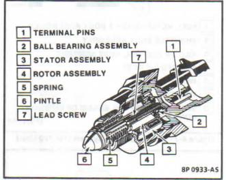
Figure 4-9 - Idle Air Control (IAC) Valve (TBI 220)
