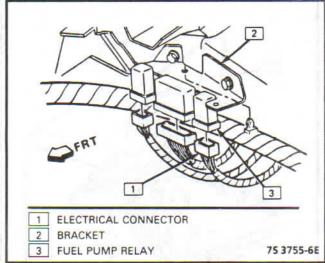
Figure 4-41 - Fuel Pump Relay (M)
