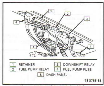
Figure 4-42 - Fuel Pump Relay (CK)
