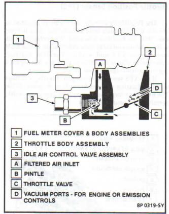
Figure 4-7 - Idle Air Control System (TBI 220 Unit)
