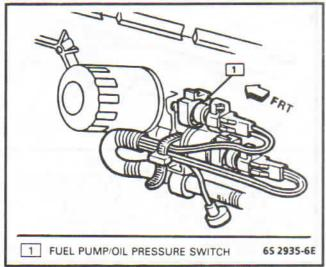
Figure 4-50 - Oil Pressure Switch (2.8L)
