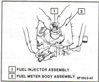
Figure 4-27 - Installing Fuel Injector - TBI 220
