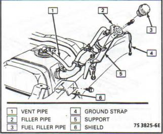
Figure 4-64 - Filler Neck - ST Chassis Cab
