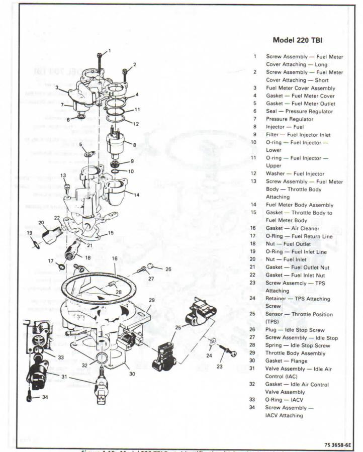
Figure 4-15 - Model 220 TBI Parts Identification (V-6 and V-8 Engine)
