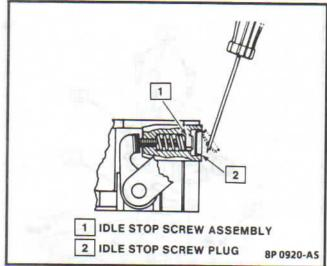
Figure 4-21 - Removing Stop Screw Plug
