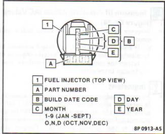
Figure 4-34 - Fuel Injector Part Number Location TBI 700
