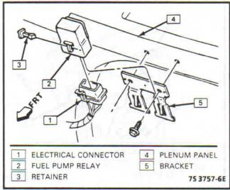
Figure 4-44 - Fuel Pump Relay (G, GP)
