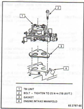
Figure 4-17 - Replacing TBI 220 Unit - 2.8L Engine
