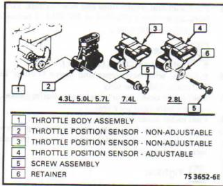
Figure 4-29 - TBI Model 220 TPS Configuration
