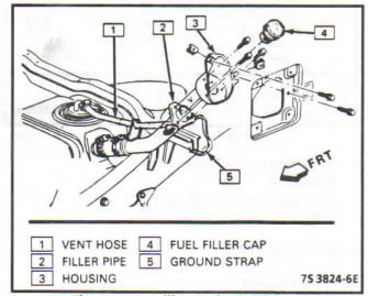
Figure 4-63 - Filler Neck - ST Pickup
