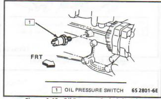
Figure 4-49 - Oil Pressure Switch (2.5L)
