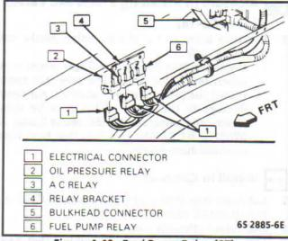
Figure 4-40 - Fuel Pump Relay (ST)
