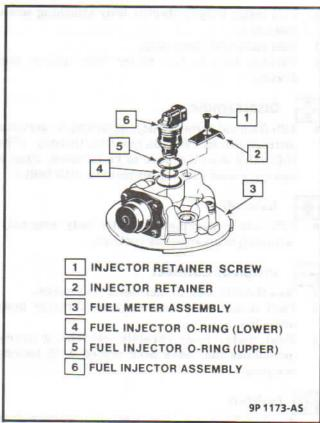
Figure 4-32 - Fuel Injection Parts (TBI 700)
