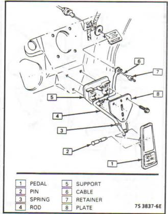
Figure 4-83 - Accelerator Pedal - M
