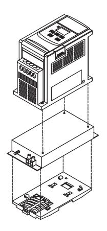
AC Drive with class B filter & Din rail mounting kit.
