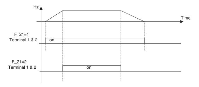
F\_22: Reverse Lockout = 0: REV run command enabled = 1: REV run command Lockout
