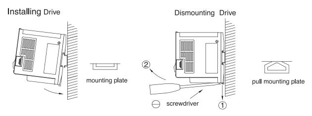
First place the groove on the back of module on the upper edge of din rail, then push the module down to lock-up position. Finally press the mounting plate upward into module.
