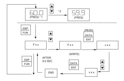
Note 1: Displays setting of frequency when stopped. Displays output frequency when running.
