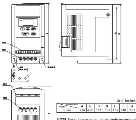
**NOTE**: For safety reasons, we strongly recommend removing the M4 grounding screw, then attach the enclosed "metal frame grounding terminal" on the same location to make a grounding bar to ensure proper grounding.
