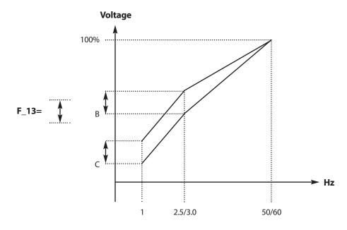
**NOTE:** When  $F_13 = 0$ , the torque boost function is disabled.
