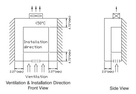
**Note:** Maximum temperature in the enclosure is 122°F (50°C) with Shield Sticker removed
