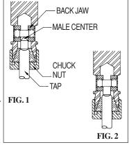
TAPPING SPEEDS: The Tapping Attachment has been designed to operate properly at recommended tapping speeds. Please refer to chart for the recommendations for specific tap sizes. **Do not exceed the maximum speed** shown on the tapping attachment.
