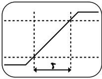
**Slew Rate Triggering.** High frequency signals with slew rates faster than expected or needed can radiate troublesome energy. Slew rate triggering surpasses conventional edge triggering by adding the element of time and allowing you to selectively trigger on fast or slow edges.
