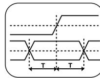
**Setup-and-Hold Triggering.** Only setup-and-hold triggering lets you deterministically trap a single violation of setup-and-hold time that would almost certainly be missed by using other trigger modes. This trigger mode makes it easy to capture specific signal quality and timing details when a synchronous data signal fails to meet setup-and-hold specifications.
