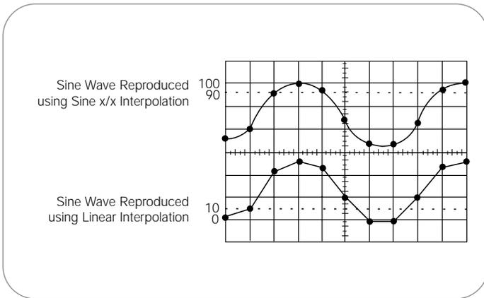
▶ **Figure 31.** Linear and sin x/x interpolation.
