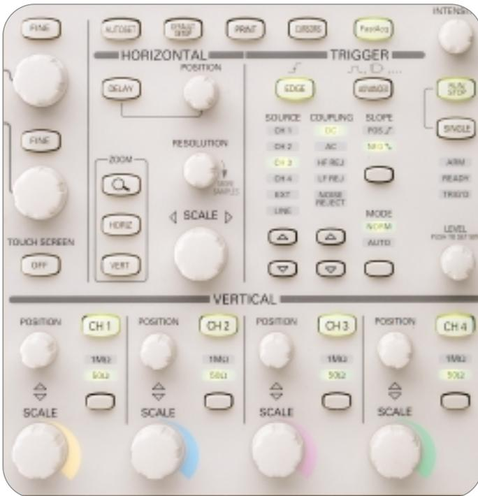
► **Figure 22.** Front-panel control section of an oscilloscope.
