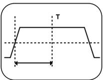
**Time-out Triggering.** Time-out triggering lets you trigger on an event without waiting for the trigger pulse to end, by triggering based on a specified time lapse.
