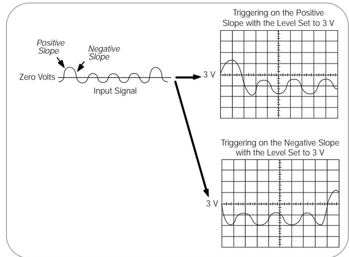
► **Figure 36.** Positive and negative slope triggering.
