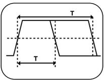
**Pulse Width Triggering.** Using pulse width triggering, you can monitor a signal indefinitely and trigger on the first occurrence of a pulse whose duration (pulse width) is outside the allowable limits.
