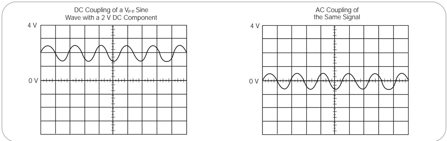
▶ **Figure 23.** AC and DC input coupling.
