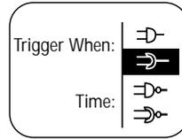
**Logic Triggering.** Logic triggering allows you to trigger on any logical combination of available input channels – especially useful in verifying the operation of digital logic.
