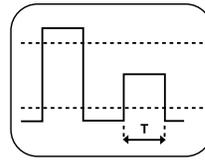
**Runt Pulse Triggering.** Runt triggering allows you to capture and examine pulses that cross one logic threshold, but not both.
