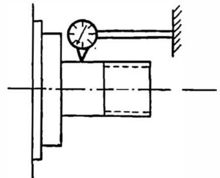
Fig. 40D. Checking a Cylinder
