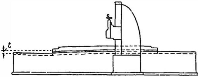
Fig. 14. Tolerances in Measuring the Difference of Height or Sag of a Planer Bed
