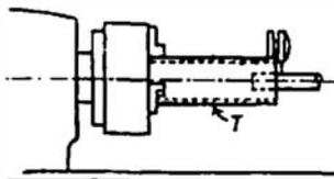
Fig. 48. Tubular Holder for Dial Gauge
