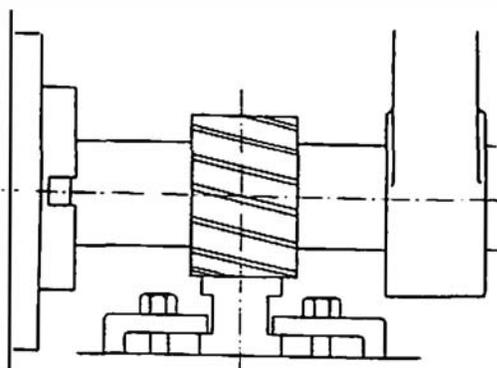
Fig. 90A. Performance Test on Milling Machine—Slab Milling
