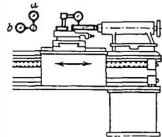
(A) IN THE CASE OF THE CENTRE LATHE, parallelism has to be checked:
