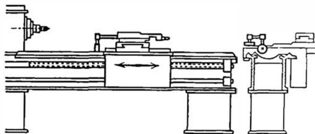
Fig. 37. Acceptance Test for Guideways
