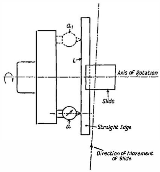
Fig. 62. Checking Perpendicularity
