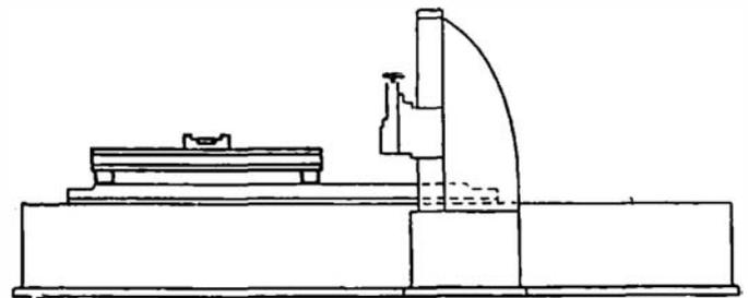
Fig. 6B. Testing Inclination of Bed with Parallels, Straight-edge and Spirit-level
