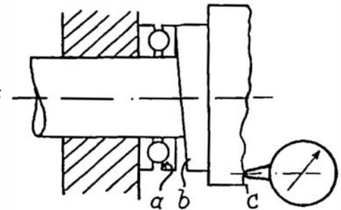
(c) External cylinders or tapers (Fig. 40B to 40D) are used for locating a chuck on a lathe spindle (Test Chart 11, Fig. 5), for locating a cutter head on a milling spindle (Test Chart 1, Fig. 2a), and for locating a grinding wheel on a grinding spindle (Test Chart 21, Fig. 11a). Tests for true running are carried out by resting the dial-gauge plunger at right angles (radially) to the surface to be tested. Readings of the dial gauge are taken while the spindle is slowly rotated.
