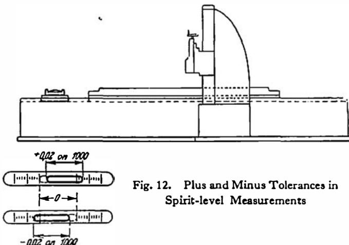
Fig. 12. Plus and Minus Tolerances in Spirit-level Measurements
