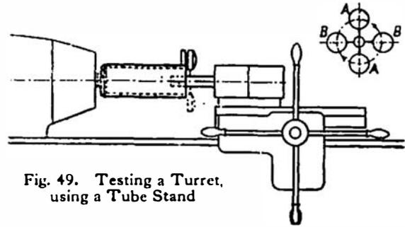
Fig. 49. Testing a Turret,
