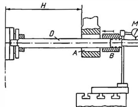
Fig. 53. Slip-bushing Method
