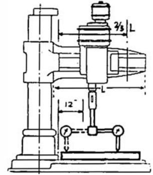
3. Perpendicularity between the feed movement of the spindle and the base plate (Test Chart 34, Figs. 7 and 8).
