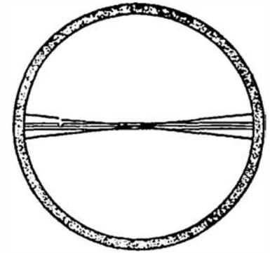
Fig. 9. Diagram showing how the Microscope Cross-wire is centred on the Taut Wire
