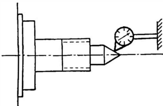
Fig. 40A. Checking the Centre
