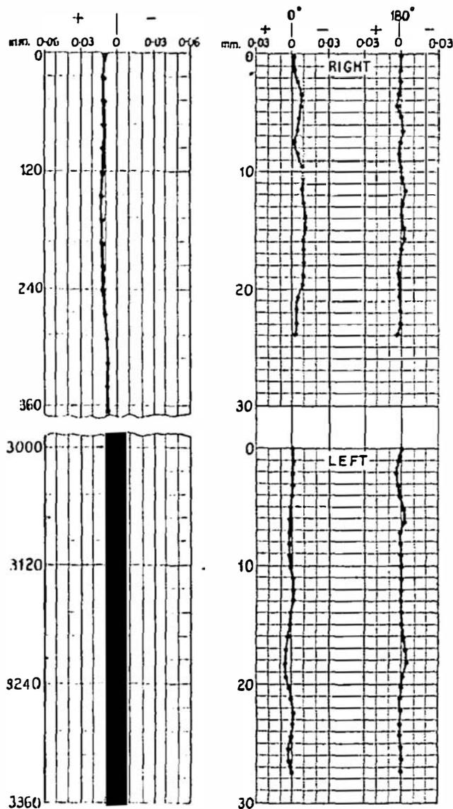
Fig. 22 (Left) Test chart for an accurate lead screw.
