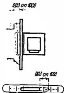
Fig. 15A. Tolerances in Testing a Surface for Flatness
