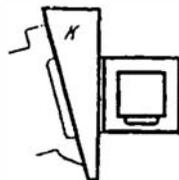
Fig. 15B. Use of an Intermediate Piece for Inclined Surfaces
