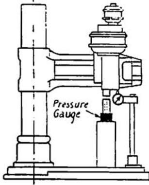
Fig. 91. Testing Vertical Thrust on Drilling Machine
