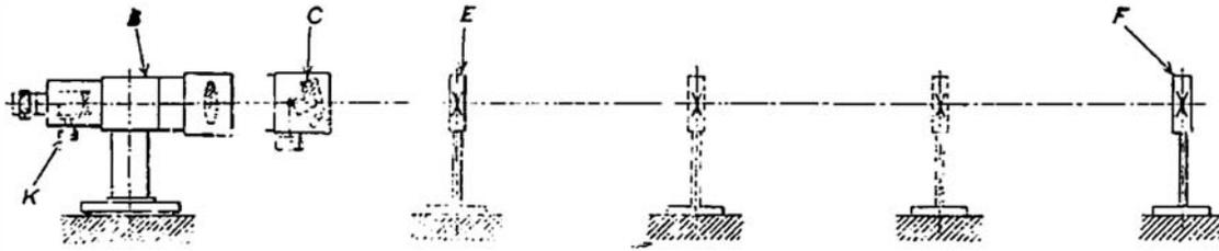
Fig. 11. General Arrangement of Optical Alignment Testing Telescope
