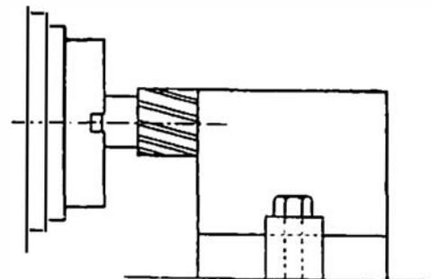
Fig. 90B. Performance Test on Milling Machine—Face Milling
