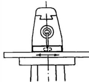
Fig. 67. Checking Parallelism of T-slot with the Table]Movement
