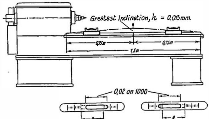
Fig. 13. Unilateral Tolerances in Spirit-level Measurements
