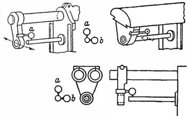
Fig. 69. Parallelism between Overarm and Spindle Axis
