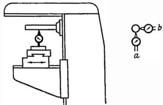
Fig. 65. Transverse Movement of Table parallel with Spindle Axis
