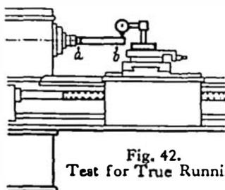
Fig. 42. Test for True Running
