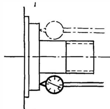
Fig. 44. Testing the Face of a Shoulder
