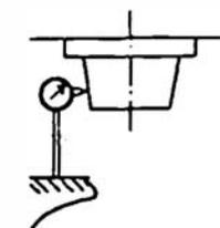
Fig. 40B. Checking a Taper
