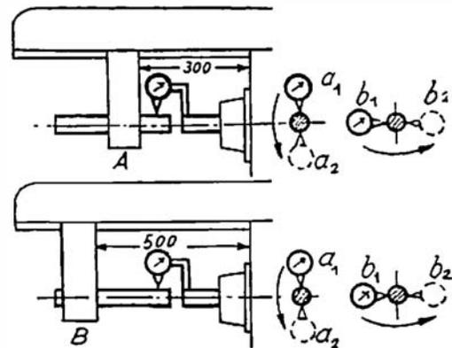
Fig. 52. Checking Spindle Alignment
