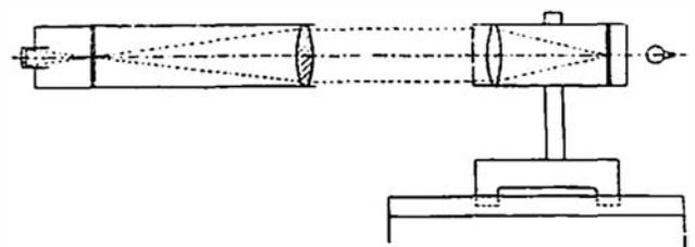
Fig. 10. Diagram illustrating the Principle of Testing by means of Target and Telescope
