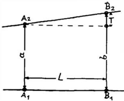
Fig. 54. Checking for Parallelism
