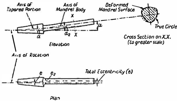
Fig. 41. Sources of Error in Rotating Mandrels
