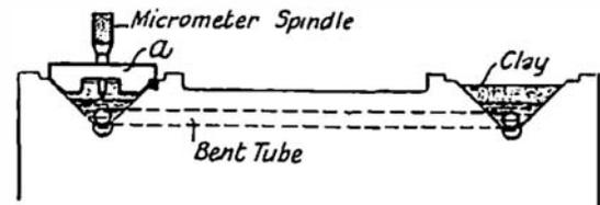
Fig. 6A. Using Vees of Bed as Water Channels when erecting Planing Machine
