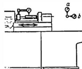
Fig. 72. Parallelism between the Spindle Axis and the Direction of the Table Traverse
