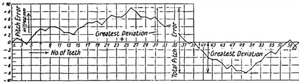
Fig. 25. Diagram of Pitch Errors of a Dividing Gear
