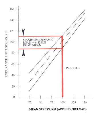
Modified Goodman diagrams help designers predict fastener performance. The broken diagonal line depicts the mean of the alternating load for a screw with a 90% probability of enduring 10 million cycles. The diagonal solid lines show that the maximum deviation of dynamic load from the mean stress is  $\pm 12$  ksi when the screw is preloaded to 100 ksi.
