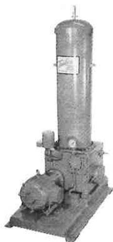
H-400 Electric-Hydraulic Barrel Pump mounts atop standard 400-lb. grease drum and has gauge, drum cover, lifting bale, 1/2 H.P. motor and adjustable pressure cut-off switch. #25550 Extension Adapter available.
