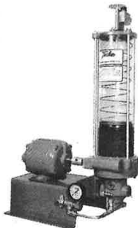
AKA Heavy-Duty Motorized Pump has internal adjustment but is usually timer-controlled. Is mounted on base with gauge, 1/4 H.P. motor and 12-lb. (or pint) or 20-lb. (or pint) grease or oil reservoir.
