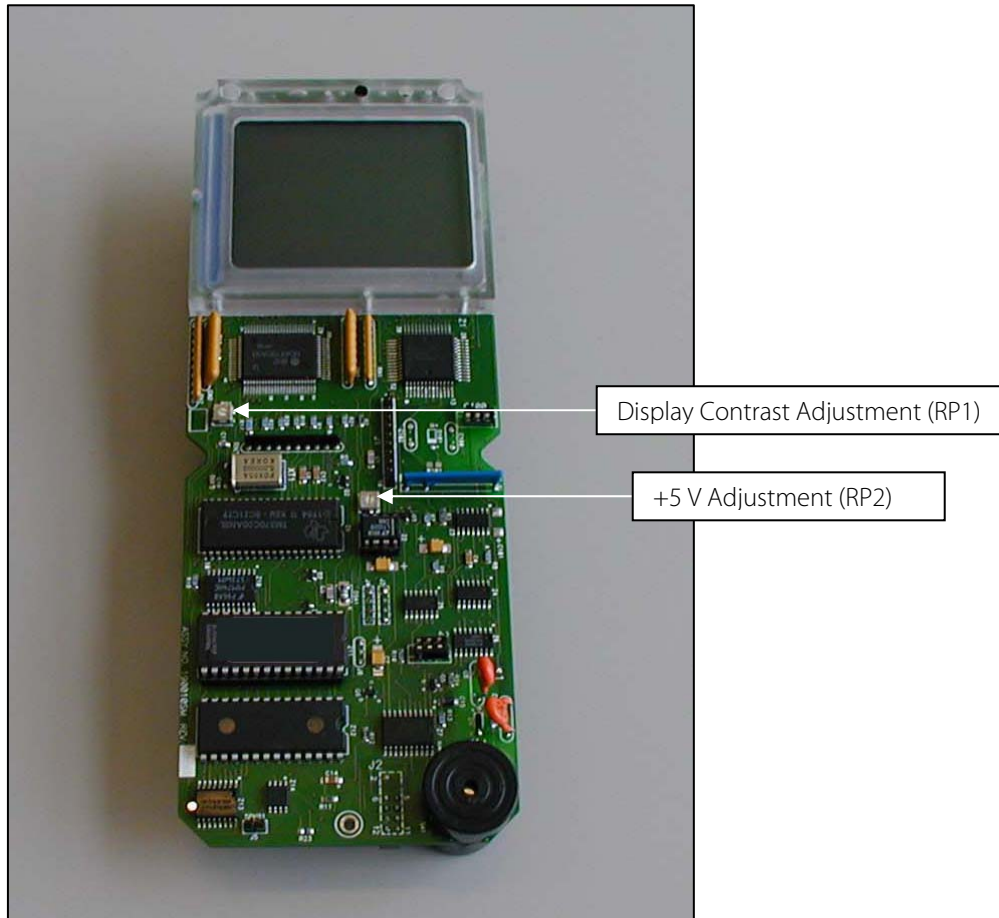
Figure 3-4. Display Contrast (RP1) and +5 (RP2) Adjustment Locations
