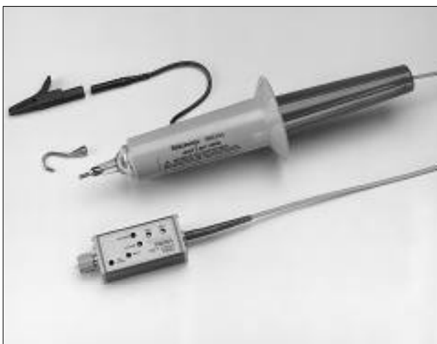
Figure 2-5. The P6015A can measure DC voltages up to 20 kV and pulses up to 40 kV with a bandwidth of 75 MHz.
