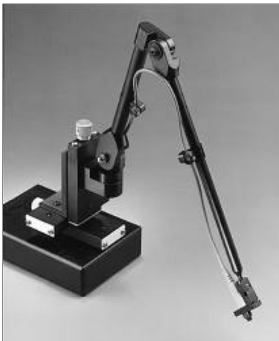
Figure 2-10. Example of a probing station designed for probing small geometry devices such as hybrid circuits and ICs.
