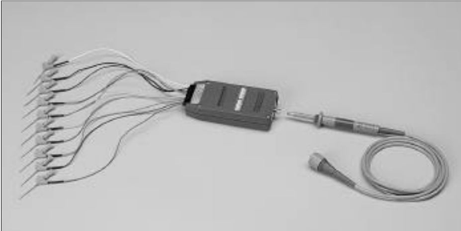
Figure 2-9. A word recognizer probe. Such probes allow oscilloscopes to be used to analyze specific data waveforms during specific logic conditions.
